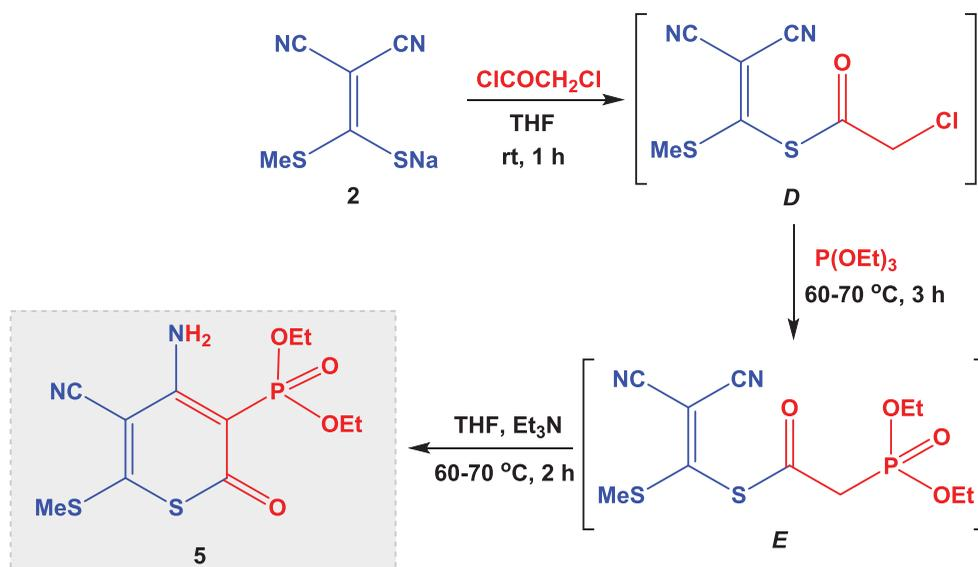
**Figure 3.** The reaction of chloroacetyl chloride with substrate **2** then with triethyl phosphite.
