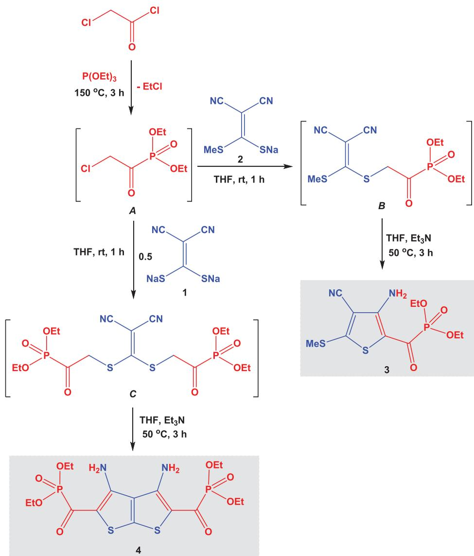
**Figure 2.** The reaction of chloroacetyl chloride with triethyl phosphite then with substrates **1** and **2**.
