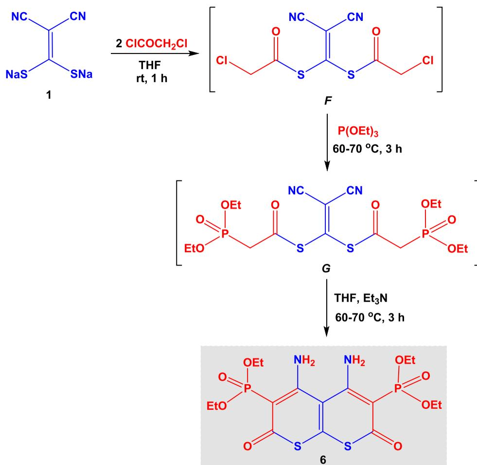
**Figure 4.** The reaction of chloroacetyl chloride with substrate **1** then with triethyl phosphite.
