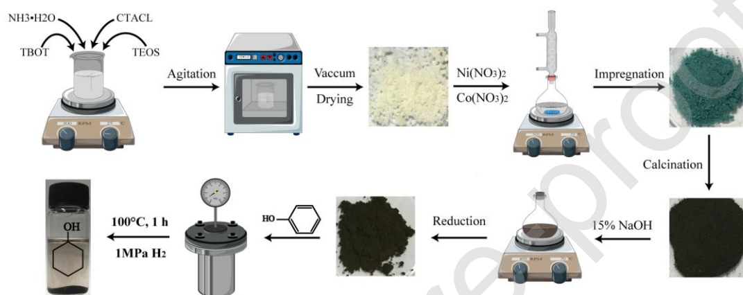
Fig. 1 Schematic of synthesis of NiCo/Si-Ti catalysts and their hydrogenation performance of phenol.
