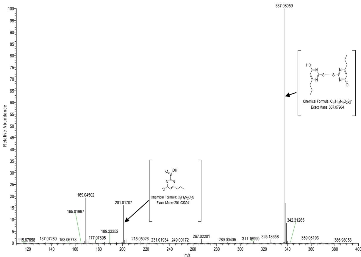
**Figure 4.** ESI-MS spectra generated with the cell potential at 400 mV.
