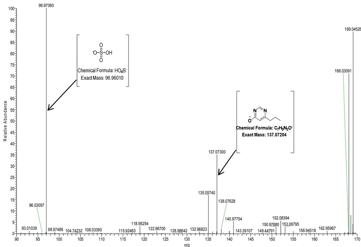
**Figure 5.** ESI-MS spectra generated with the cell potential at 800 mV.
