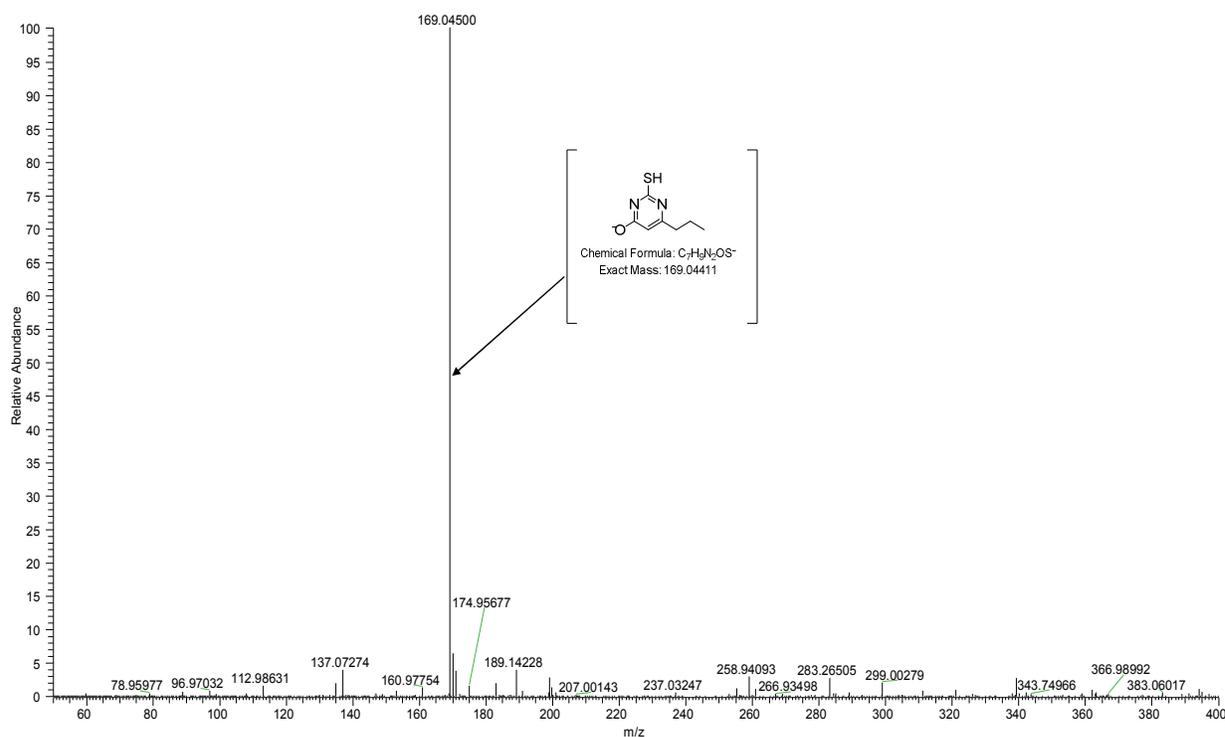
**Figure 3** ESI (-) MS, with cell turned off 0 mv obtained for 0.1 mM PTU in 20 mM ammonium phosphate buffer, 20% MeOH, pH 10, Flow rate 10  $\mu$ L/min.
