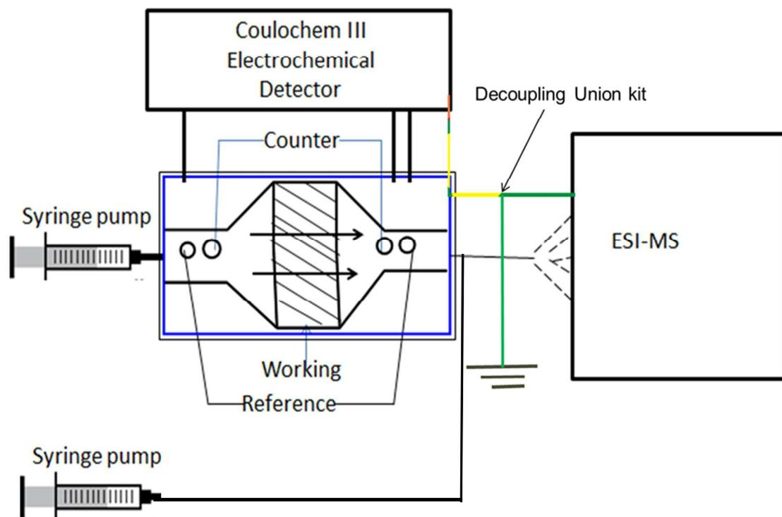
**Figure 2.** Schematic of EC/ESI –MS system. Coulochem III Electrochemical Detector controls potential of the flow through cell. Samples were infused at 10  $\mu\text{L}/\text{min}$ .
