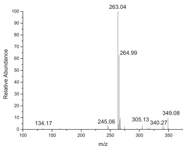
FIGURE 2 Mass spectrum of clenproperol
