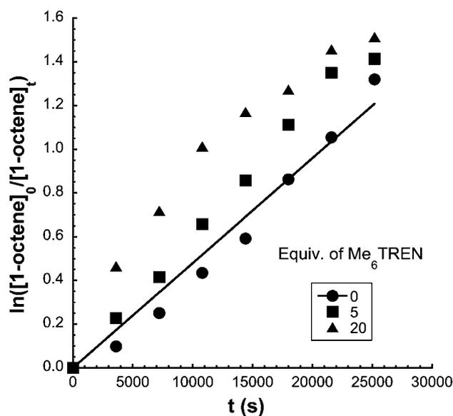
**Fig. 3** First order kinetic plots for ATRA of 1-octene to  $\text{CCl}_4$  catalyzed by  $[\text{Cu}^{\text{II}}(\text{Me}_6\text{TREN})\text{Cl}][\text{Cl}]$  in the presence of 0 (●), 5 (■), and 20 (▲) equivalents of free  $\text{Me}_6\text{TREN}$ .  $T = 60^\circ\text{C}$ , solvent =  $\text{CH}_3\text{CN}$ ,  $[\text{1-octene}]_0 : [\text{CCl}_4]_0 : [\text{AIBN}]_0 : [\text{Cu}^{\text{II}}]_0 = 5000 : 5500 : 250 : 1$ ,  $[\text{1-octene}]_0 = 1.34\text{ M}$ .
