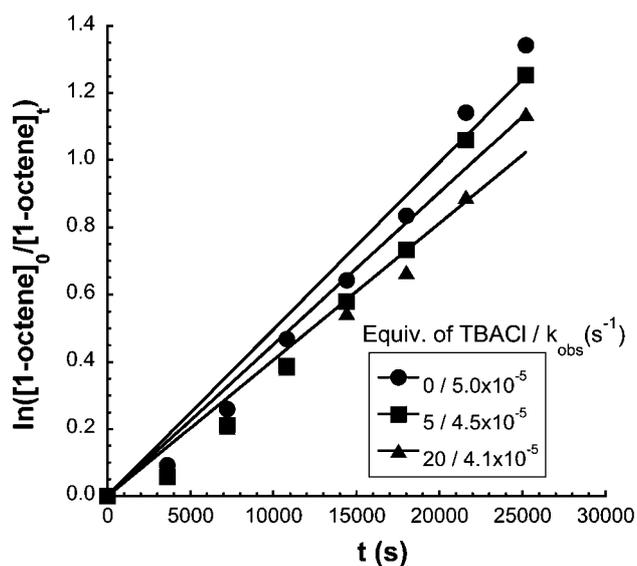
**Fig. 4** First order kinetic plots for ATRA of 1-octene to  $\text{CCl}_4$  catalyzed by  $[\text{Cu}^{\text{II}}(\text{Me}_6\text{TREN})\text{Cl}][\text{Cl}]$  in the presence of 0 (●), 5 (■), and 20 (▲) equivalents of TBACl.  $T = 60^\circ\text{C}$ , solvent =  $\text{CH}_3\text{CN}$ ,  $[\text{1-octene}]_0 : [\text{CCl}_4]_0 : [\text{AIBN}]_0 : [\text{Cu}^{\text{II}}]_0 = 5000 : 5500 : 250 : 1$ ,  $[\text{1-octene}]_0 = 1.34\text{ M}$ .
