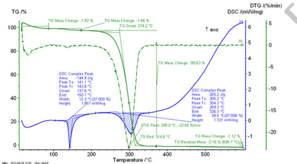
**Figure 3.** DSC, TG, and TDG curves of compound **4a2**.
