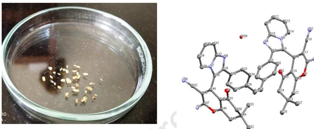
Figure 3: a) Crystals of 7i compound b) ORTEP diagram of 7i (CCDC 1865906)
