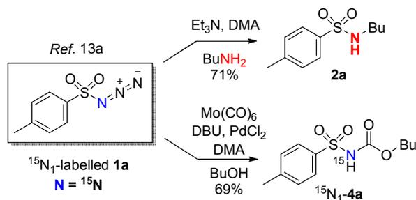
**Scheme 3.** Mechanistic investigation using  $^{15}\text{N}_1$ -labeled **1a**
