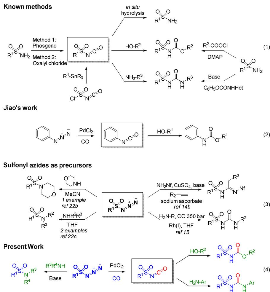
**Scheme 1.** Synthesis of sulfonylamides, sulfonyl carbamates and sulfonyl ureas.
