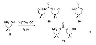
18 was chosen to examine the effect of steric bulk at the position  $\beta$  to the nucleophilic nitrogen and the Thorpe–Ingold effect of the *gem*-dimethyl substituents at C3. Accordingly, the carbamate was expected to be favored by the presence of the *gem*-dimethyl
