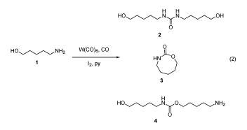
reaction conditions of a substrate concentration of 4 M, 40  $^{\circ}$ C, 80 atm CO and a reaction time of 18 h afforded the bis-(hydroxyalkyl)urea 2 in 64% yield and the cyclic carbamate 3 in only 2% yield. The acyclic carbamate 4 was not detected in the reaction mixtures. However, the presence of unreacted starting material was observed by TLC prior to purification of the products.
