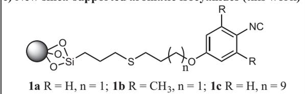
**Scheme 1.** Soluble, supported and new isocyanide-based scavengers for Ru removal from catalytic reactions such as ring-closing metathesis (RCM).
