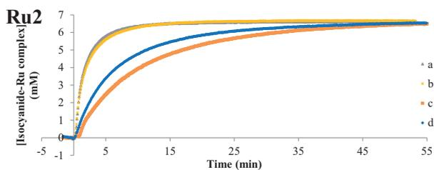
**Fig. 2.** In situ FTIR analysis of Ru carbene binding by solution-phase isocyanides. Entries a, b, c, and d correspond to reactions of **4a** at 23.5 °C, **4b** at 23.5 °C, **4a** at 0 °C, and **4b** at 0 °C.
