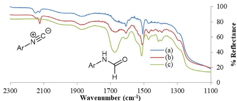
**Fig. 1.** DRIFT IR of silica gel material **1a** produced by grafting at (a) 25 °C, 94% isocyanide, (b) 80 °C, 45% isocyanide, and (c) silica-supported formamide, **5a**.
