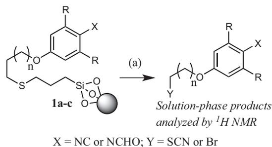
Conditions: (a) 1) crushed 4 Å mol. sieves, CD<sub>3</sub>CN, rt, overnight;
