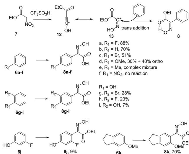
**Scheme 2.** Mechanism of benzaldoxime formation in superacid from ethyl nitroacetate and aromatics for the preparation of scaffold **8**. Compounds **8a,b,d,k** already reported in Ref. **38**. For **8a** the yields have been improved with a new procedure.
