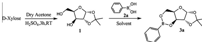
**Scheme 1.** Synthesis of 1,2-*O*-isopropylidene- $\alpha$ -D-xylofuranose-3,5-phenyl boronate **3a** from D-xylose.
