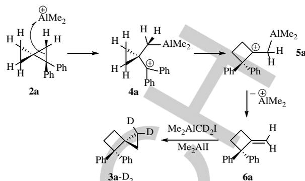
**Scheme 4.** Proposed mechanism for the transformation of spiro[2.2]pentanes into spiro[2.3]hexanes.
