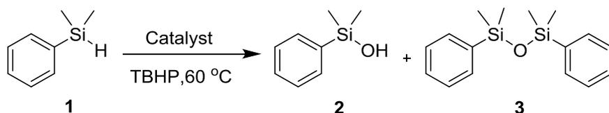
Scheme 1. Oxidation of silane into silanol using TBHP or water as oxidant in the presence of MOFs as heterogeneous solid catalysts.
