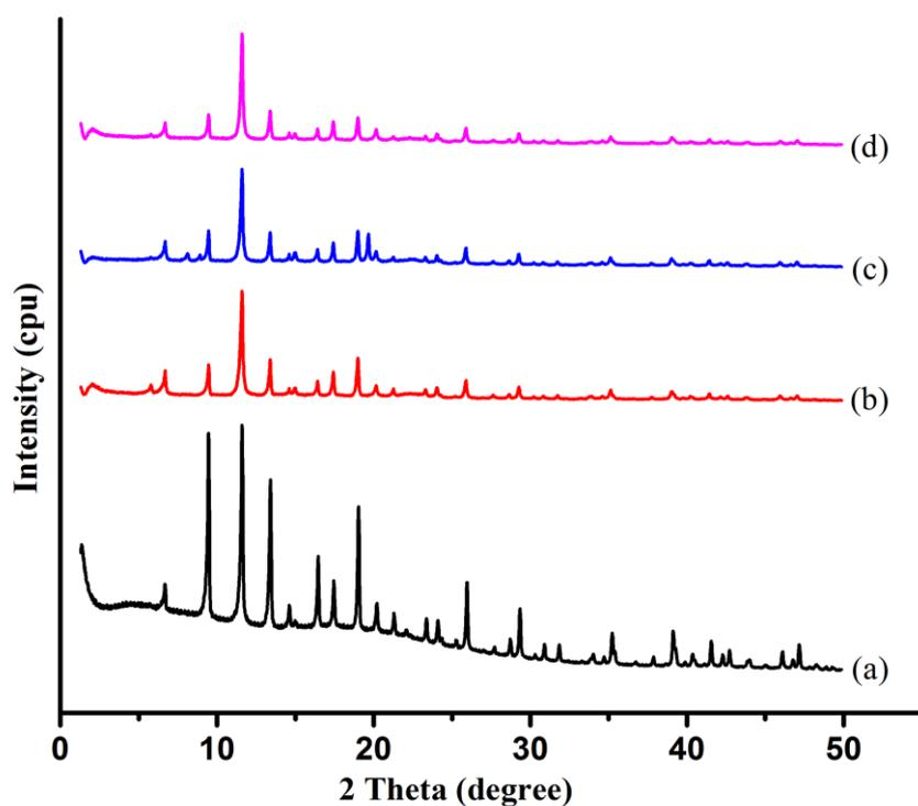
Figure 3. Powder XRD pattern of (a) fresh, (b) the recovered MOF after the reaction of **1** with TBHP, (c) the recovered MOF from triphenylsilane with TBHP and (d) the recovered catalyst from diphenylsilane with TBHP  $\text{Cu}_3(\text{BTC})_2$ .
