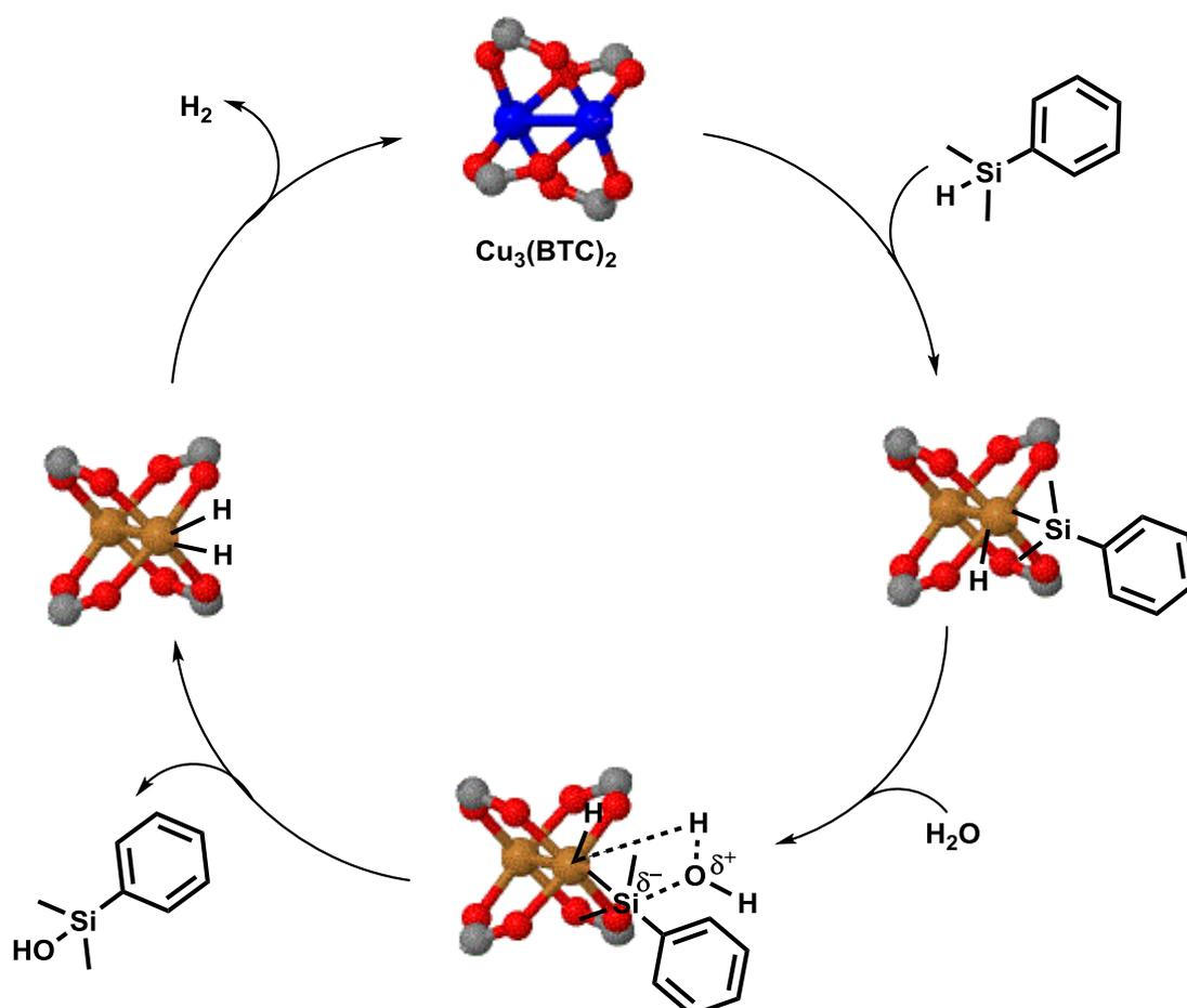
**Scheme 2.** A proposed mechanism for the oxidation of **1** to **2** with water using  $\text{Cu}_3(\text{BTC})_2$  as heterogeneous solid catalyst.
