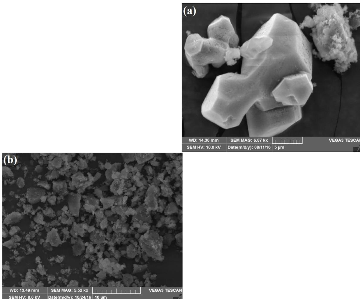
Figure 5. SEM images of (a) fresh and (b) the recovered  $\text{Cu}_3(\text{BTC})_2$  after the reaction of **1** with TBHP.
