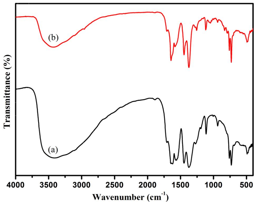
Figure 4. FT-IR spectrum of (a) fresh and (b) the recovered  $\text{Cu}_3(\text{BTC})_2$  after the reaction of **1** with TBHP.
