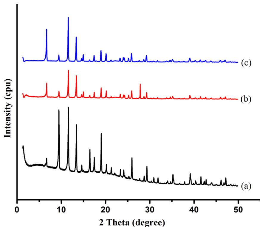
Figure 8. Powder XRD pattern of Cu<sub>3</sub>(BTC)<sub>2</sub> (a) fresh, (b) recovered after the reaction of **1** with H<sub>2</sub>O, (c) recovered after the reaction of diphenylsilane with H<sub>2</sub>O.
