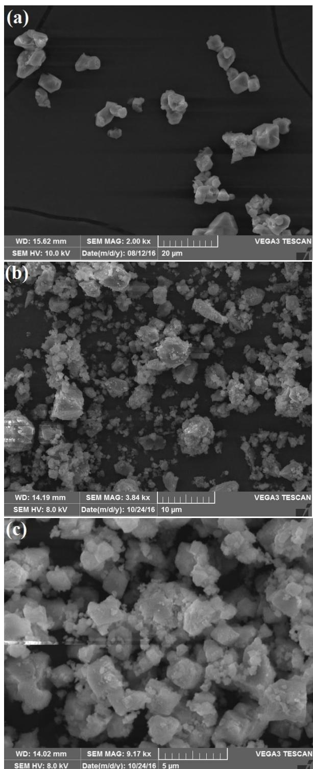
Figure 10. SEM images of (a) fresh, (b) recovered after the reaction of **1** in water and (c) four times used  $\text{Cu}_3(\text{BTC})_2$ .
