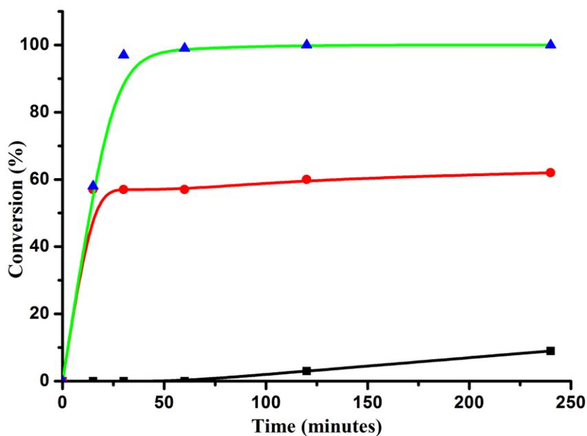
Figure 7. Leaching test for the oxidation of **1** to **2**. In the presence of catalyst (▲), the catalyst filtered after 15 minutes (●) and the poison test with pyridine under the optimized conditions (■). Reaction conditions: **1** (1 mmol),  $\text{H}_2\text{O}$  (20 mmol), THF (1 mL) and  $\text{Cu}_3(\text{BTC})_2$  (25 mg), 65 °C, 4 h.
