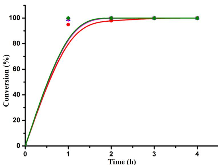
Figure 6. Reusability of  $\text{Cu}_3(\text{BTC})_2$  as heterogeneous solid catalyst for the oxidation of **1** to **2** using water as oxidant. Reaction conditions: **1** (1 mmol),  $\text{H}_2\text{O}$  (20 mmol), THF (1 mL) and  $\text{Cu}_3(\text{BTC})_2$  (25 mg), 65 °C, 4 h.
