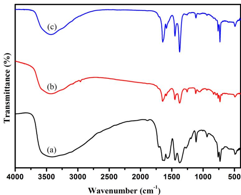
Figure 9. FTIR spectrum of (a) fresh, (b) recovered after the reaction from **1** and (c) four times used Cu<sub>3</sub>(BTC)<sub>2</sub>.
