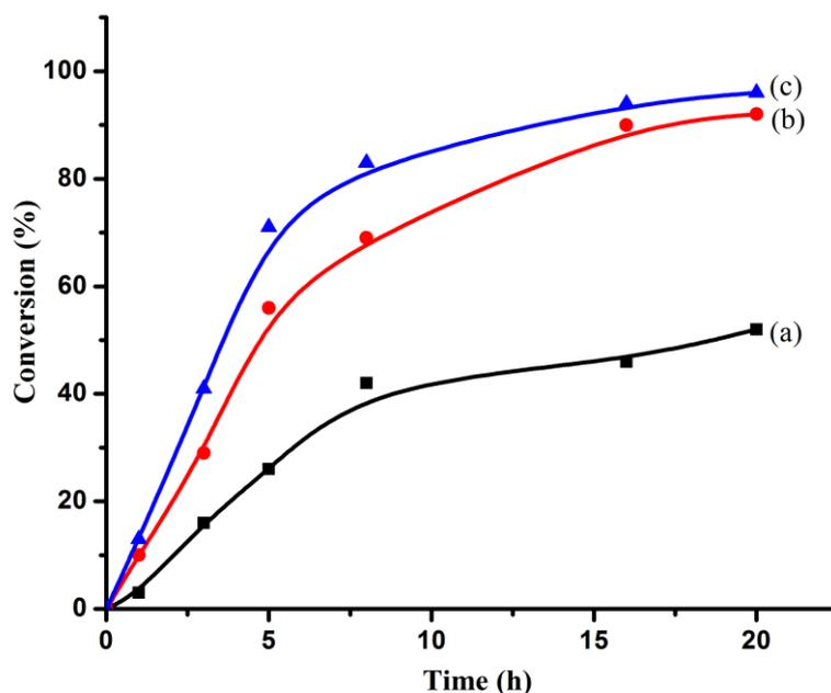
Figure 1. Time conversion plot for the conversion of **1** using  $\text{Cu}_3(\text{BTC})_2$  as heterogeneous solid catalyst with (a) 1, (b) 2 and (c) 3 mmol of TBHP as oxidant. Reaction conditions: **1** (1 mmol), TBHP (mmol),  $\text{Cu}_3(\text{BTC})_2$  (25 mg), 60 °C.
