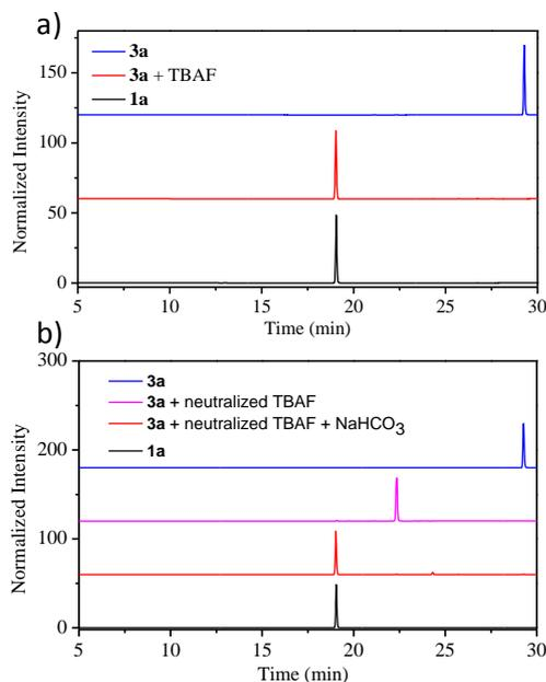
**Figure 1.** Deprotection of **3a** by TBAF monitored by HPLC. a) HPLC trace of reaction mixture of **3a** and TBAF (red line) in THF for 0.5 h at 310 nm. b) HPLC trace of reaction mixture of **3a** and neutralized TBAF (pH 7) before (magenta line) and after treatment with NaHCO<sub>3</sub> (aq.) (red line). See Supplementary Information for details.
