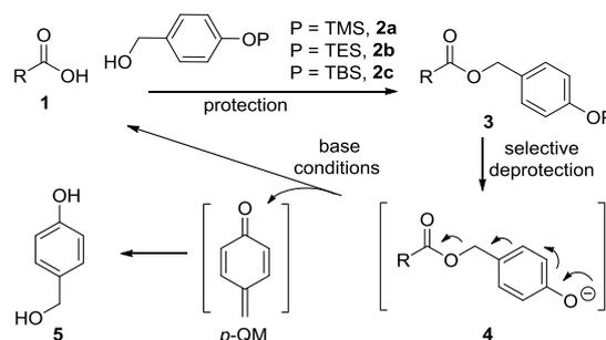
Scheme 1. Protection of carboxylic acid with caged 4-hydroxyl benzyl.
