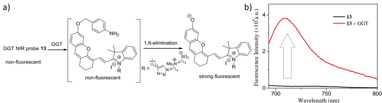
**Figure 2.** a) GGT-mediated cleavage of probe **13** and turn-on of fluorescence; b) Fluorescent spectra of probe **13** before (black line) and after incubation with GGT (red line). λ<sub>ex</sub> = 682 nm.
