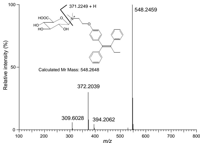
Fig. 2. Representative mass spectrum of TAM  $N^+$ -glucuronides formed from TAM by human liver microsomes. The spectrum was taken at the retention time of 9.4 min in Fig. 1A.
