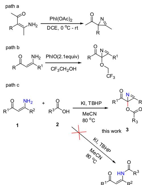
**Scheme 1.** Existing methods for construction of  $\alpha$ -substituted 2*H*-azirines from enamines.
