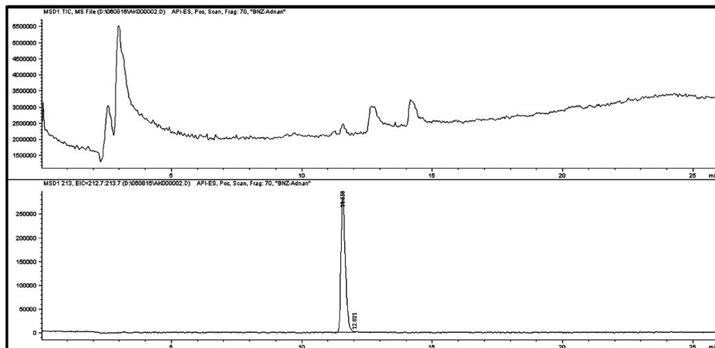
**Figure 4.** TIC and SIM ( $m/z$  213) chromatograms of 30 min RLM incubation with HIE-124 (**4**).
