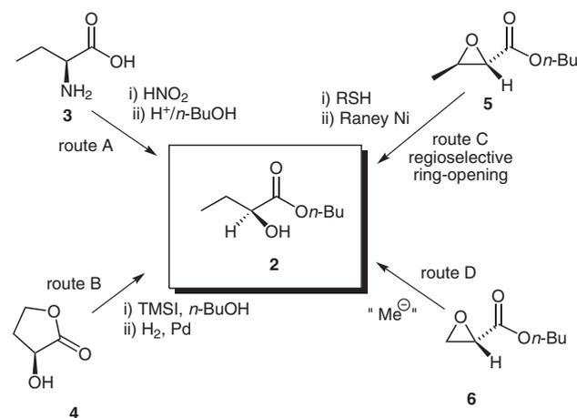
**Scheme 2** Four synthetic approaches for production of butyl (*S*)-2-hydroxybutanoate (**2**)
