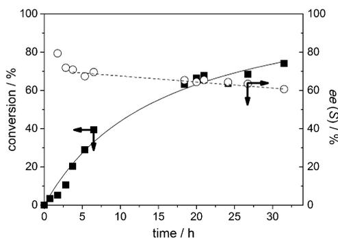
**Figure 1.** Conversion and enantiomeric excess values of the enzymatic synthesis of  $\alpha,\alpha$ -difluoroacetophenone cyanohydrin. Reagents and conditions: two-phase system consisting of diisopropyl ether/50 mM citrate phosphate buffer pH 5 (1:1), substrate (50 mM), hydrogen cyanide (250 mM), MeHNL (133 U mL<sup>-1</sup>), 10 °C.
