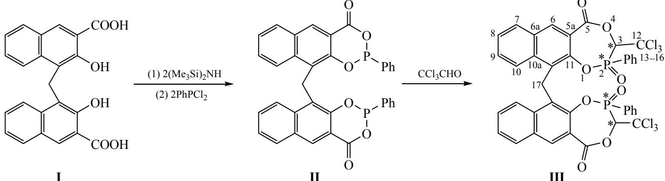
Compound **II** reacts with the prochiral chloral under mild conditions with the formation of six stereoisomeric bis(naphtho-1,4,2-dioxaphosphepines) (**III**) ( $\delta_p$  33.6, 32.5, 31.6, 31.2, 29.3, 28.7 ppm) in the ratio 4:5:5:33:4:9. This reaction gives rise to four chiral center resulting in the formation of a mixture of
