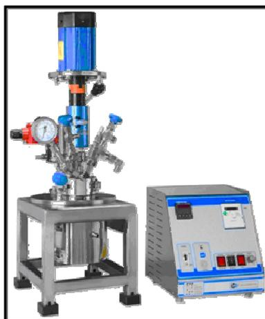
**Fig. 1** High Pressure Reactor.
