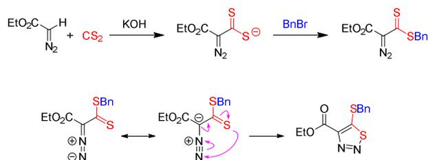
In summary, we have developed an operationally simple method for the synthesis of 4,5-disubstituted 1,2,3-thiadiazoles via the nucleophilic addition of  $\alpha$ -diazo carbonyl compounds to carbon disulfide. This method can be applied as an alternative to traditional synthesis methods of 1,2,3-thiadiazoles with carbon disulfide as the C1 building block with mild reaction conditions.
