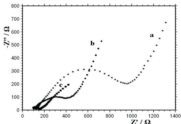
Fig. 2. Electrochemical impedance spectra for (a) Nafion/Hb-CPE, (b) Nafion/Hb-CILE, (c) Nafion/CILE in the presence of 10.0 mmol L<sup>-1</sup> [Fe(CN)<sub>6</sub>]<sup>3-/4-</sup> and 0.1 mol L<sup>-1</sup> KCl with the frequencies swept from 10<sup>5</sup> to 0.05 Hz.
