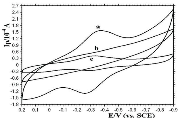
Fig. 3. Cyclic voltammograms of (a) Nafion/Hb-CILE, (b) Nafion/CILE and (c) Nafion/Hb-CPE in pH 7.0 PBS at the scan rate of  $100 \text{ mV s}^{-1}$ .
