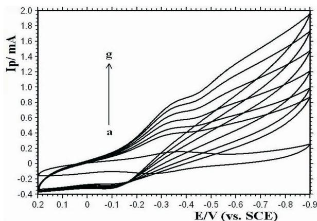
Fig. 5. Cyclic voltammograms of Nafion/Hb-CILE in pH 7.0 PBS before (a) and after the addition of 38.0, 48.0, 72.0, 100.0, 124.0, 128.0  $\text{mmol L}^{-1}$  of TCA (curve b-g), respectively, at the scan rate of 100  $\text{mV s}^{-1}$ .
