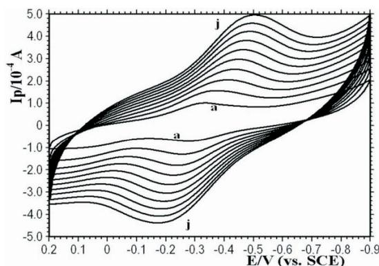
Fig. 4. Cyclic voltammograms of Nafion/Hb-CILE with different scan rates (from a to j: 50, 100, 150, 200, 250, 300, 350, 400, 450,  $500 \text{ mV s}^{-1}$ ) in pH 7.0 PBS.
