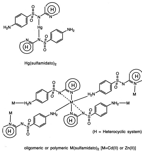
Proposed structures of M(sulfamidato)<sub>2</sub> in DMSO solution
