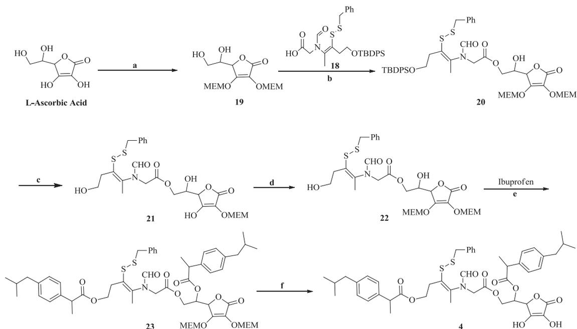
**Scheme 4.** The synthetic route of prodrug **4**. Reagents and conditions: (a) MEMCl, DIEA, DCM, r.t., 1 h; (b) intermediate acid **18**, DCC, DMAP, r.t., overnight; (c) 50% AcOH, 50 °C, 3.5 h; (d) MEMCl, DIEA, DCM, r.t., 1 h; (e) ibuprofen, DCC, DMAP, DCM, r.t., overnight; (f) 1% HCl–EtOH, 70 °C, 1 h.
