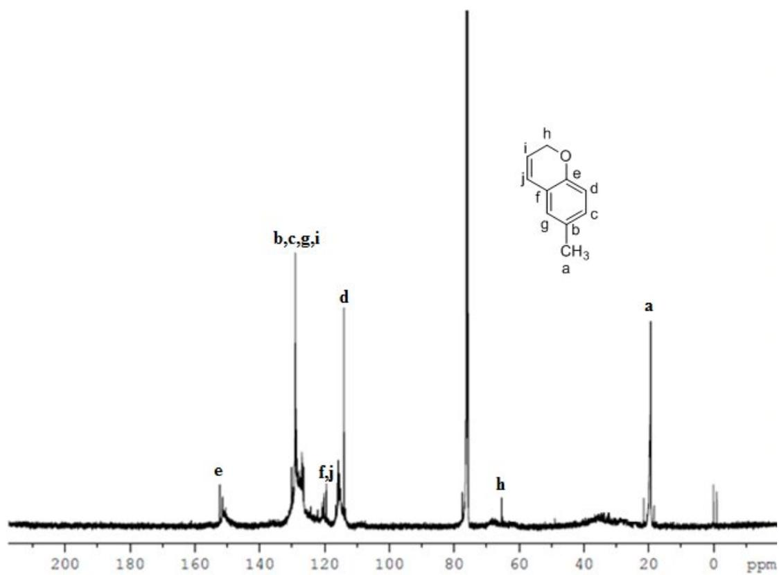
$^{13}\text{C}$  NMR spectrum of cured MPPR (solvent :  $\text{CDCl}_3$ )
