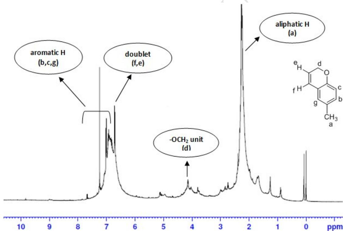
$^1\text{H}$  NMR spectrum of cured MPPR (solvent :  $\text{CDCl}_3$ )
