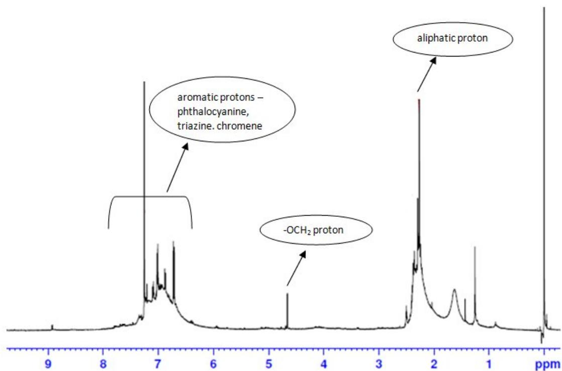
$^1\text{H}$  NMR spectrum of cured blends (CMPPN-MPPR) (solvent :  $\text{CDCl}_3$ )
