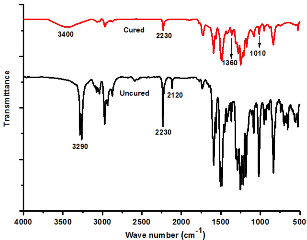
Fig. 4. FT-IR spectra of 1.5BPhPN-PR and its cured form C1.5 BPhPN-PR (330 °C, 5 h)
