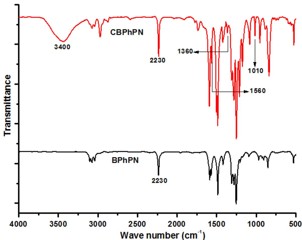
**Fig 2.** FT-IR spectra of BPhPN monomer and its cured form CBPhPN
