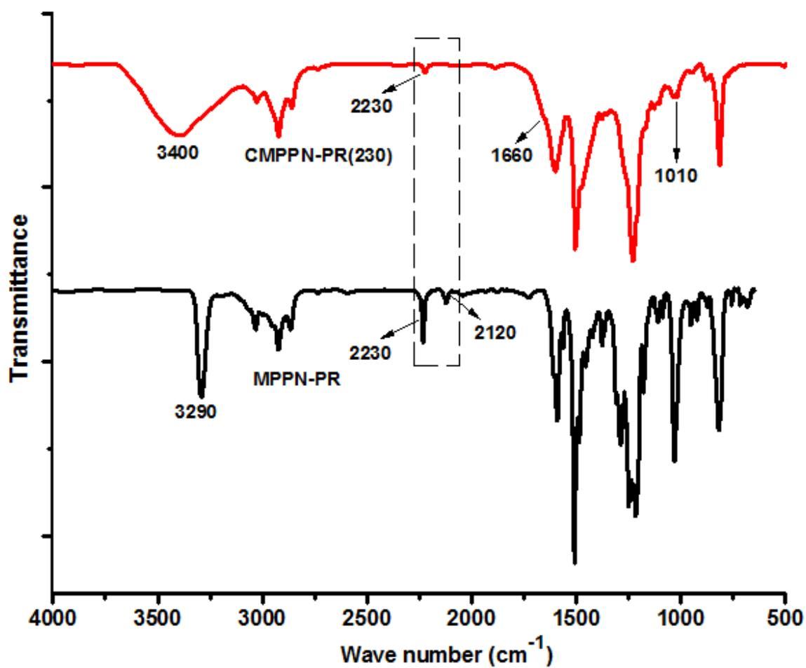
Fig. 3. FT-IR spectra of blends of model compounds MPPN-PR and its cured form
