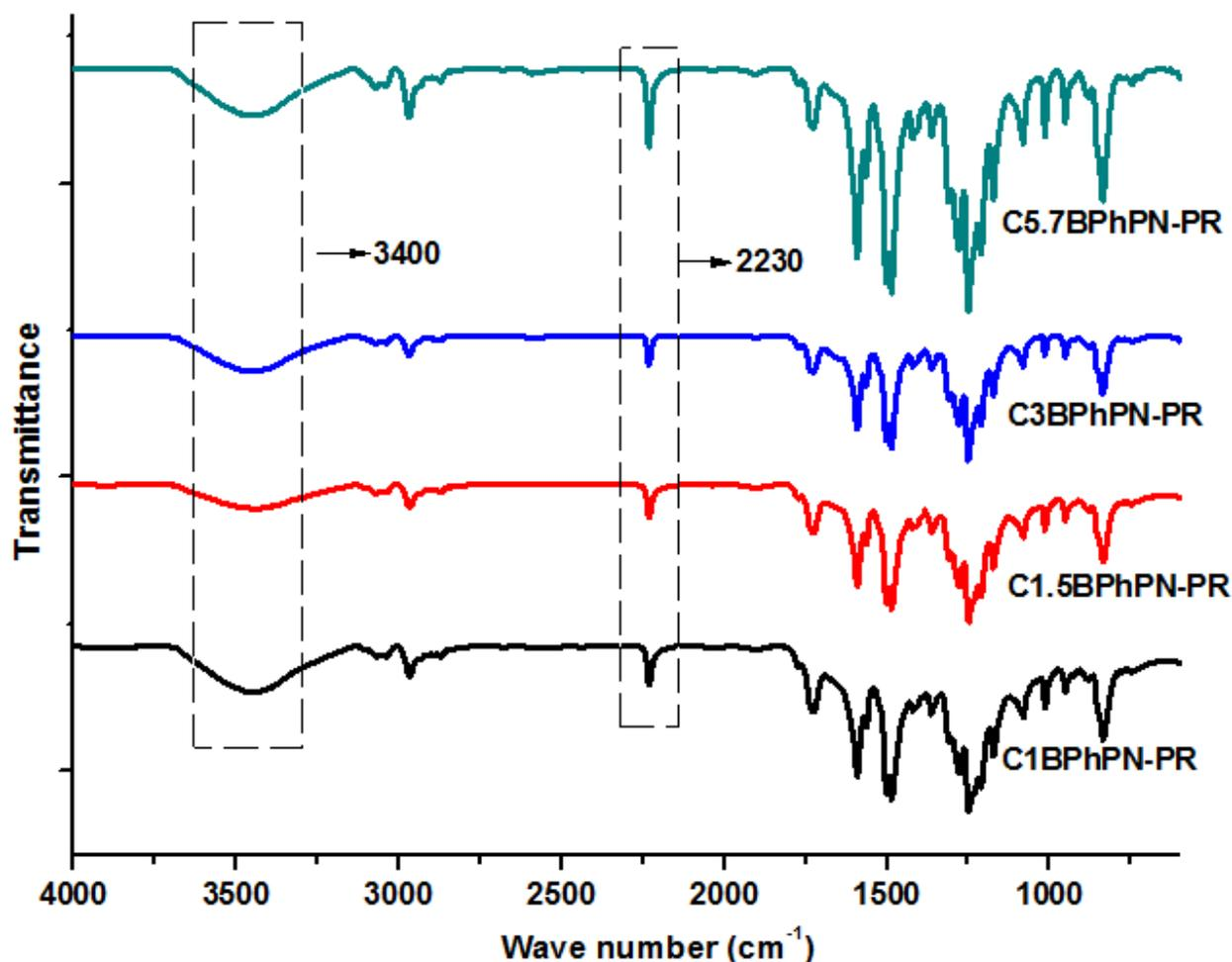
**Fig. 5** FT-IR spectra of cured BPhPN-PR blends (330 °C, 5 h)
