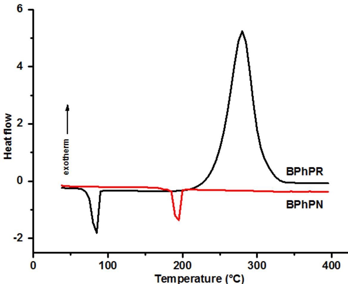
**Fig.8a.** DSC profile of bisphthalonitrile and bispropargyl monomers
