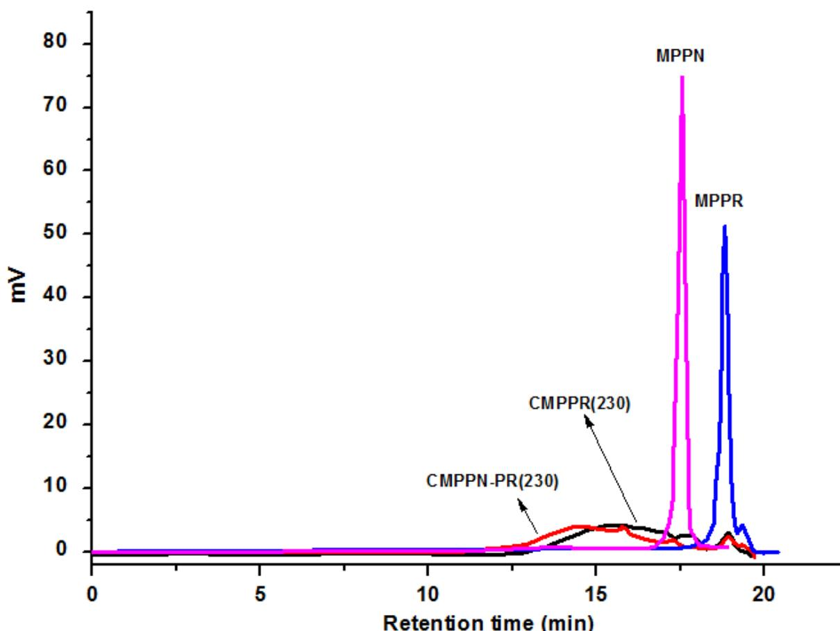
Fig.11. GPC chromatogram of model compounds and their cured forms
