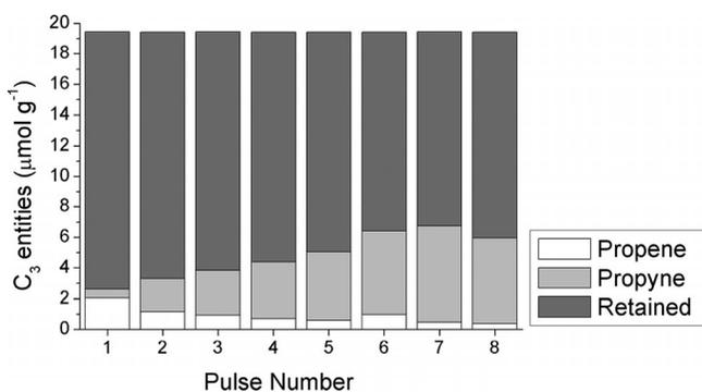
**Figure 3.** Carbon mass balance profile for the Au(azide)/Al<sub>2</sub>O<sub>3</sub> catalyst after reduction/pre-treatment at 663 K then propyne hydrogenation reaction testing at 523 K.
