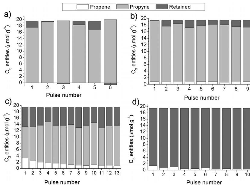
**Figure 1.** Carbon mass balance profiles corresponding to propyne hydrogenation over the Au(azide)/Al<sub>2</sub>O<sub>3</sub> catalyst at the following reaction temperatures: (a) 323 K, (b) 423 K, (c) 523 K, and (d) 623 K. The catalyst was reduced at 523 K prior to reaction testing in all cases.
