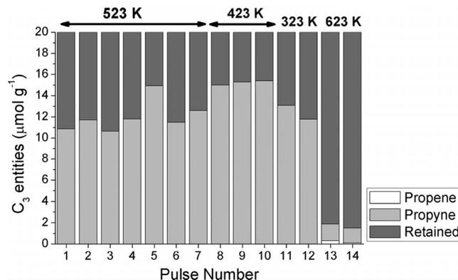
**Figure 2.** Carbon mass balance profile for propyne hydrogenation over alumina at a range of temperatures: pulses 1–7, 523 K; pulses 8–10, 423 K; pulses 11–12, 323 K and pulses 13–14, 623 K. The alumina was exposed to a reduction treatment at 523 K prior to reaction testing.
