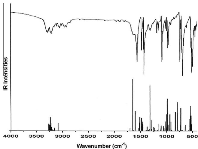
**Fig. 2.** The experimental (upper) and the calculated non-scaled (lower) vibrational spectra of complex **1a**.
