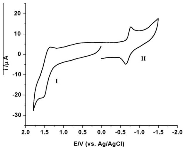
Fig. 4. CV of **1a** in dichloromethane at a scan rate of 100 mV s<sup>-1</sup>. The analyte concentration was 0.97 × 10<sup>-3</sup> M.
