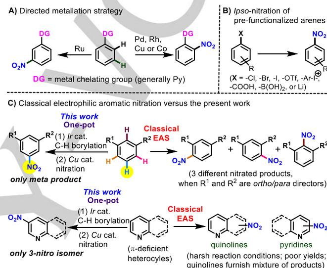
**Scheme 1.** [A] Regioselective aromatic nitration using metallation strategies. [B] *ipso*-nitration of suitably pre-functionalized arenes. [C] Comparison of the present work with the classical electrophilic aromatic nitration method.
