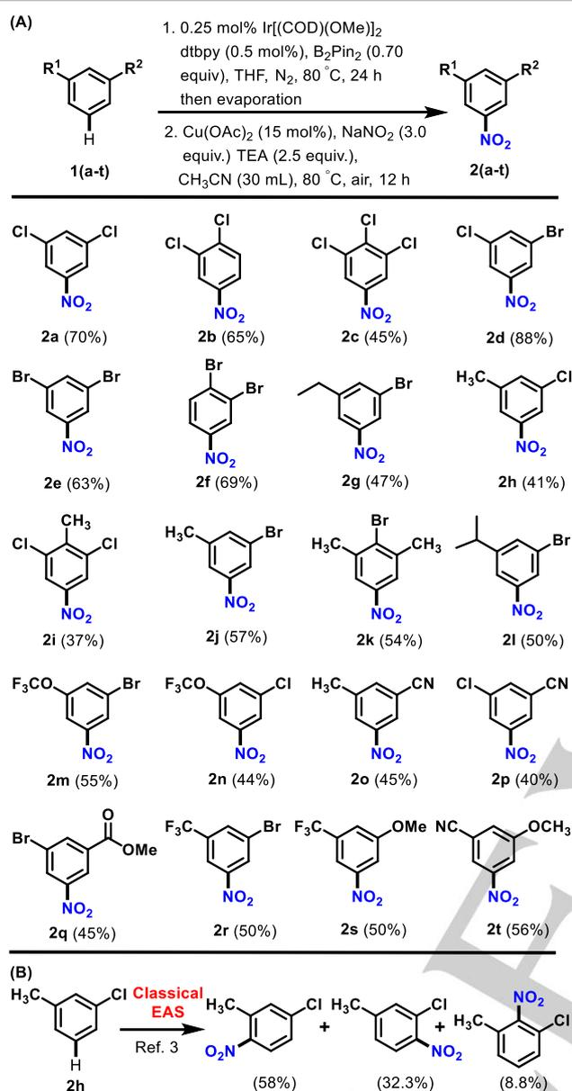
**Table 2.** [A] Scope of arenes in the C-H borylation/nitration sequence. Reactions were performed on 1.0 mmol scale. [B] Classical nitration on **2h**
