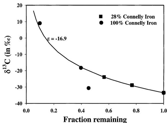
Fig. 3. Carbon isotopic composition of TCE versus fraction of TCE remaining during reductive dechlorination by Connelly zero-valent cast iron in column experiments in Experiment 3. Error bars represent 0.5‰ accuracy and reproducibility and are smaller than plot symbols. The line represents a Rayleigh model curve based on an enrichment factor of  $-16.9‰$  determined from all data using Eq. (3) (see text).
