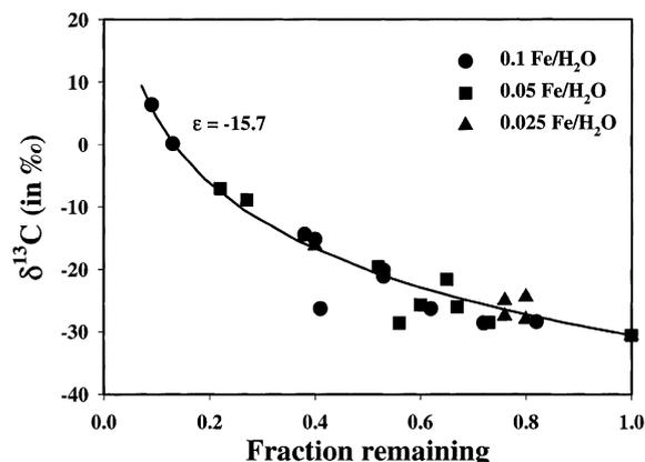
Fig. 1. Carbon isotopic composition of TCE versus fraction of TCE remaining during reductive dechlorination by Peerless zero-valent cast iron at three different iron/water ratios in Experiment 1. Error bars represent 0.5‰ accuracy and reproducibility and are smaller than plot symbols. The line represents a Rayleigh model curve based on an enrichment factor of  $-15.7\%$  determined from all data using Eq. (3) (see text).
