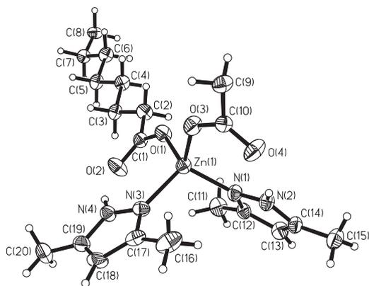
**Fig. 11.** Molecular structure of complex **6** showing the atomic numbering scheme at 30% ellipsoid probability level.
