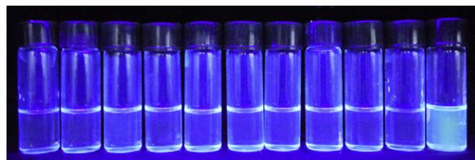
**Fig. 4.** Photographs of **1** in DMF treated with different metal ions at  $1.0 \times 10^{-4}$  M ( $\text{Cd}^{2+}$ ,  $\text{Co}^{2+}$ ,  $\text{Cr}^{3+}$ ,  $\text{Cu}^{2+}$ ,  $\text{Mn}^{2+}$ ,  $\text{Ni}^{2+}$ ,  $\text{Pb}^{2+}$ ,  $\text{Hg}^{2+}$ ,  $\text{Fe}^{2+}$ ,  $\text{Fe}^{3+}$  and  $\text{Zn}^{2+}$ , from left to right).
