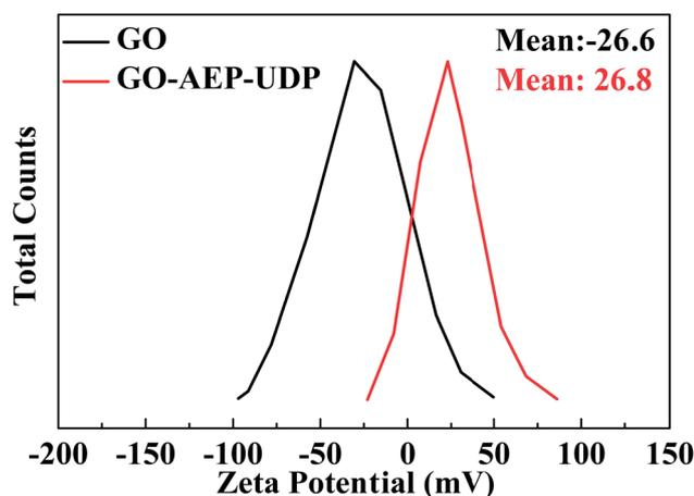
Fig. 4 The zeta potentials of GO and GO-AEP-UDP.
