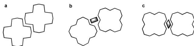
**Figure 8.** Simplified, two-dimensional model of packing for a less spherical (a) and a more spherical (b and c) four-fold substituted molecule. Guest molecules included in the packing are shown as dark objects.
