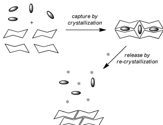
**Scheme 2.** Uptake of a hazardous or unstable small molecule into a crystalline phase of TDA and subsequent recovery of the TDA carrier material by addition of a volatile solvent in the form of re-crystallization that leaves the small molecule in the solution with the solvent.
