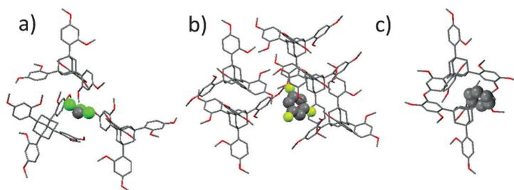
**Figure 4.** Structural details from inclusion complexes of **3** in triclinic crystal systems with a) chloroform (only one of the guest molecules is shown), b) 1,3,5-trifluorobenzene, and c) benzene as guests. Hydrogens were omitted for clarity. Color code: Carbon, grey; oxygen, red; chlorine, green; fluorine, light green. See Table 2, entries 11, 16, and 23 for further details.
