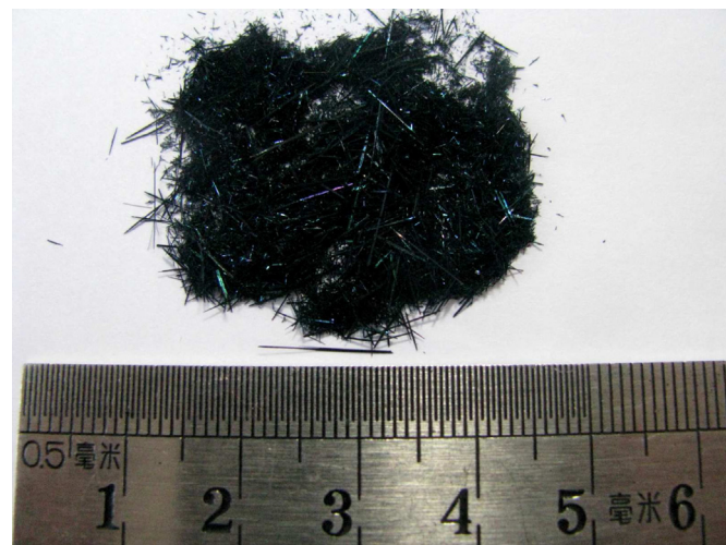
Fig. 1. Optical micrograph of as prepared MnPc crystals synthesized at 190 °C for 3 h.
