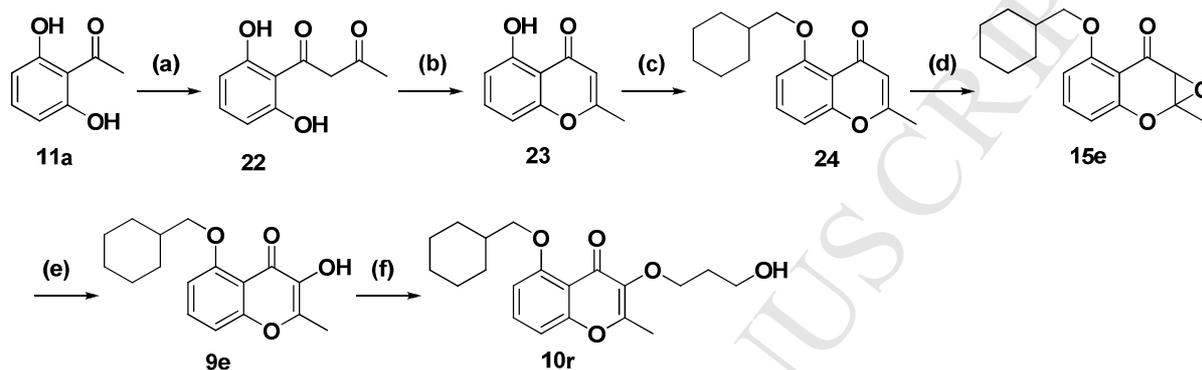
**Scheme 4.** Synthesis of 2-methyl chromen-4-one derivative **10r**. Reagents and Conditions: (a) Na, EtOAc, rt, 18 h; (b) MeOH, Conc.HCl, 60 °C, 2 h, 75%; (c) Cy-CH<sub>2</sub>-Br,  $K_2CO_3$ , DMF, 60 °C, 16 h, 65%; (d) mCPBA, EtOH/DCM (1:1), rt, 24 h, 32%; (e) Acetone, Conc.HCl, rt, 16 h, 68%; (f) OH-(CH<sub>2</sub>)<sub>3</sub>-Br,  $K_2CO_3$ , DMF, 60 °C, 16 h, 55%.
