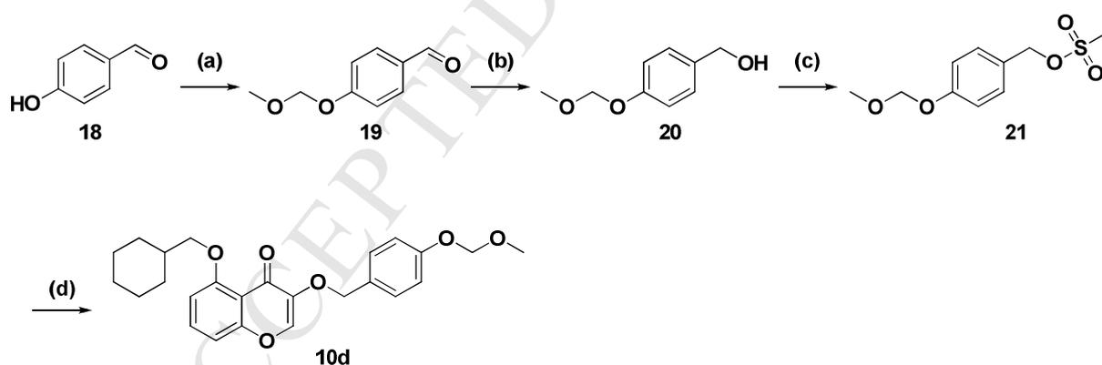
**Scheme 3.** Synthesis of chromen-4-one derivative **10d**. Reagents and Conditions: (a) MOM-Cl, 60% NaH, DMF, 0 °C, 30 min, 92%; (b) NaBH<sub>4</sub>, methanol, 0 °C, 30 min, 90%; (c) CH<sub>3</sub>SO<sub>2</sub>Cl, TEA, DCM, 0 °C to rt, 1 h, 85%; (d) Compound **9a**, K<sub>2</sub>CO<sub>3</sub>, DMF, 20 °C, 24 h, 55%.
