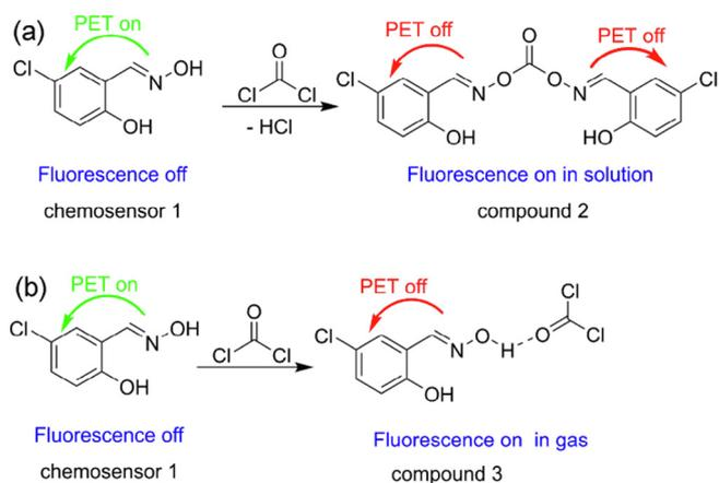
**Fig. 6.** The proposed detection mechanisms of chemosensor 1 towards phosgene in solution (a) and gas phase (b).
