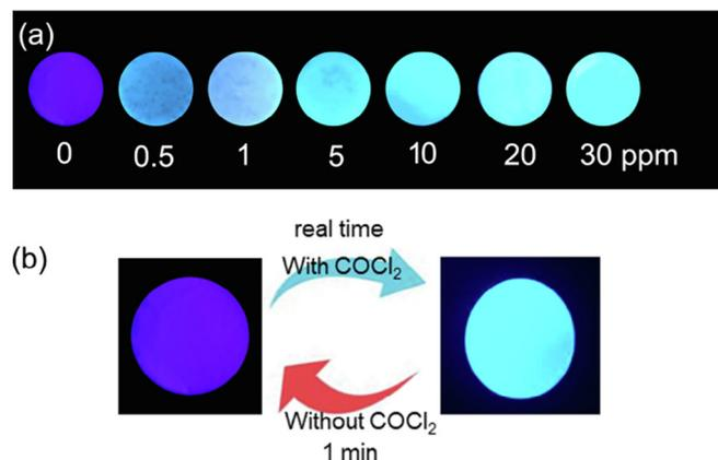
**Fig. 5.** (a) Color change of chemosensor test papers upon exposure to various amounts of phosgene vapor. (b) A reversible process for detecting phosgene with test papers.
