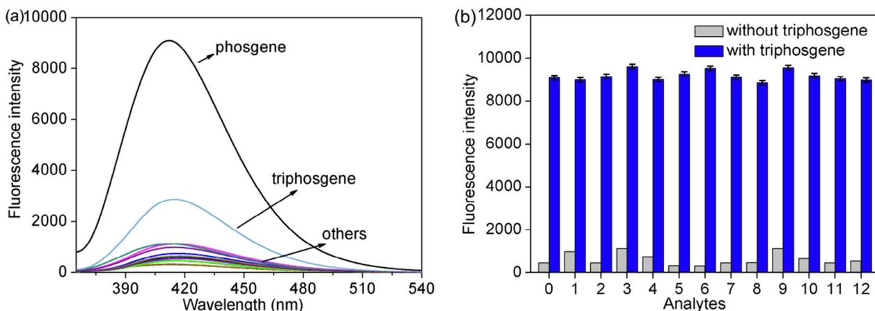
**Fig. 3.** (a) Selectivity and (b) specificity of chemosensor 1 (50  $\mu\text{M}$ ) to triphosgene (240  $\mu\text{M}$ ) and other analytes (240  $\mu\text{M}$ ). (1)  $\text{SOCl}_2$ , (2)  $\text{POCl}_3$ , (3) acetyl chloride, (4) Dimethylaminozoyl chloride, (5) TFA, (6) HCl, (7) 2,4-Dinitrobenzenesulfonyl chloride, (8) Oxalyl chloride, (9) paratoluensulfonyl chloride, (10) Oxalyl hydrazine, (11) bisacrylamide, (12) DCP.
