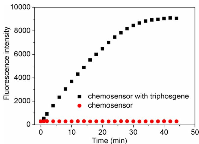
**Fig. 4.** Change in the fluorescence intensity (410 nm) of chemosensor 1 (50  $\mu\text{M}$ ) after the addition of triphosgene (240  $\mu\text{M}$ ).
