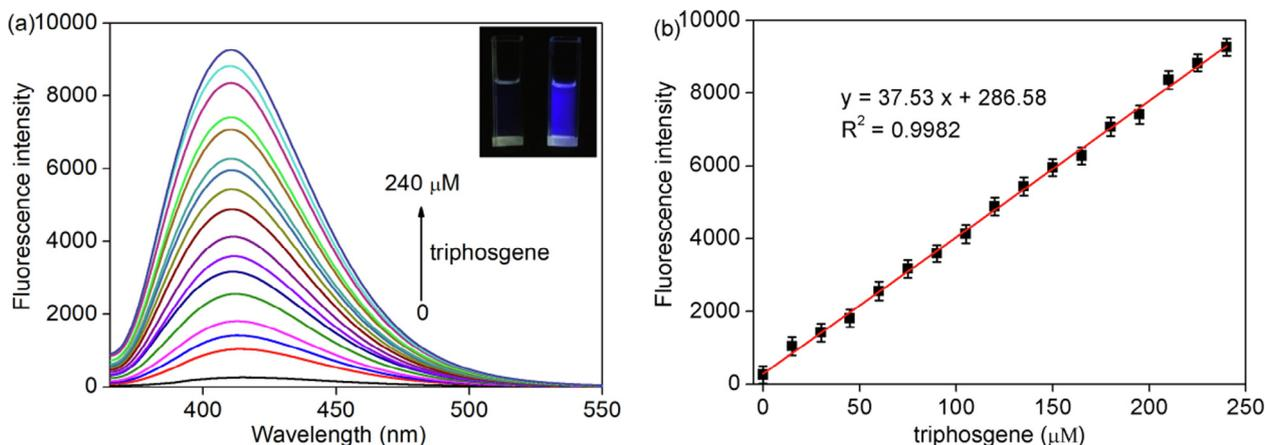
**Fig. 2.** (a) Fluorescence spectra of chemosensor 1 (50  $\mu\text{M}$ ) in  $\text{CH}_2\text{Cl}_2$  (containing 0.1% TEA, v/v) along with the addition of various amounts of triphosgene. (b) Linearity between the fluorescence intensity (410 nm) of chemosensor 1 (50  $\mu\text{M}$ ) and concentration of triphosgene (0–240  $\mu\text{M}$ ).
