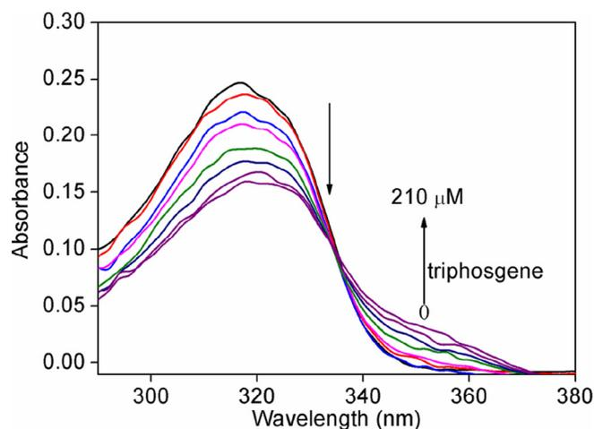
Fig. 1. UV–vis spectra of chemosensor 1 (50  $\mu\text{M}$ ) in  $\text{CH}_2\text{Cl}_2$  (containing 0.1% TEA, v/v) along with the addition of triphosgene (0–210  $\mu\text{M}$ ).
