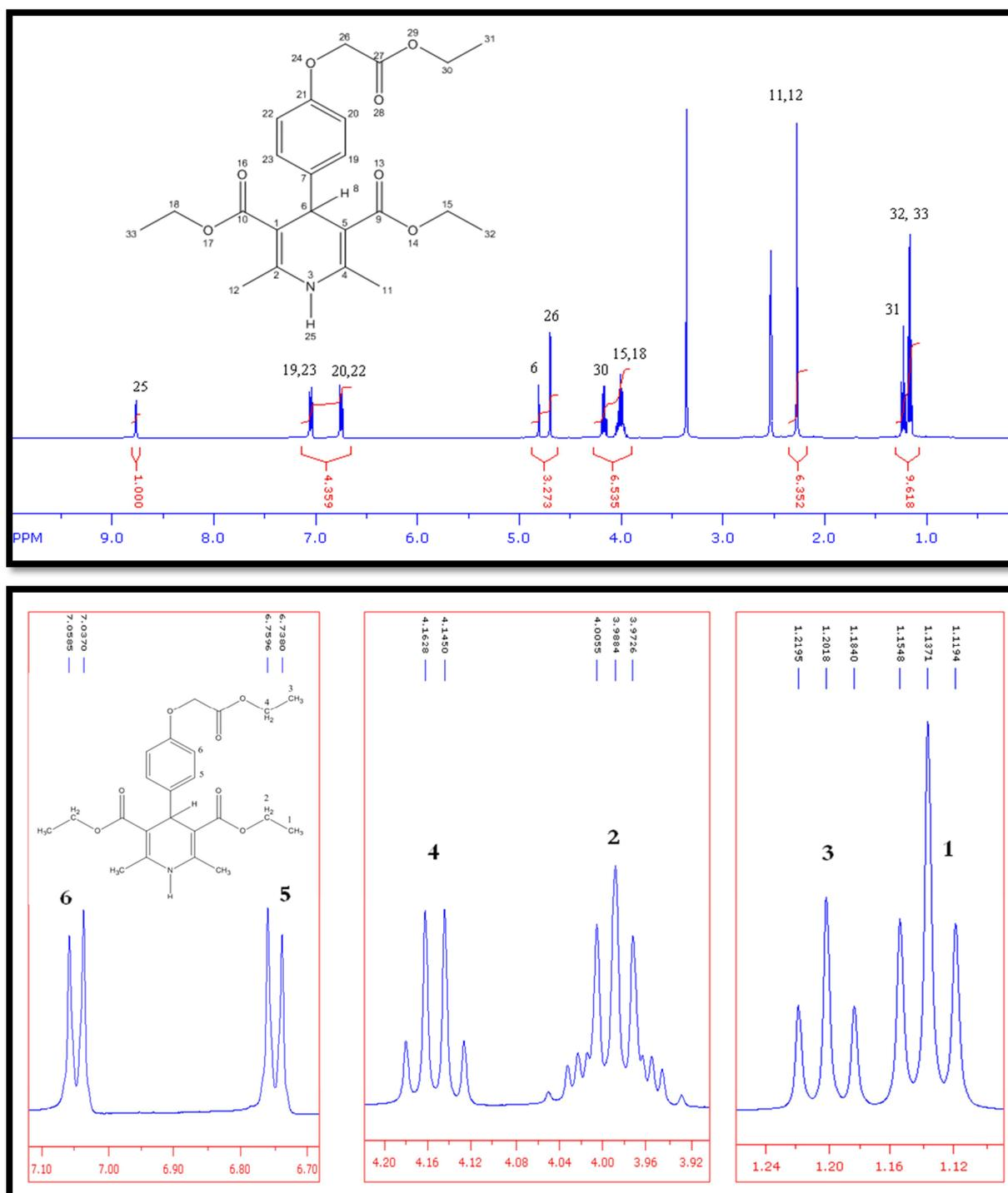
**Figure 3.**  $^1\text{H}$  NMR spectra of compound 2
