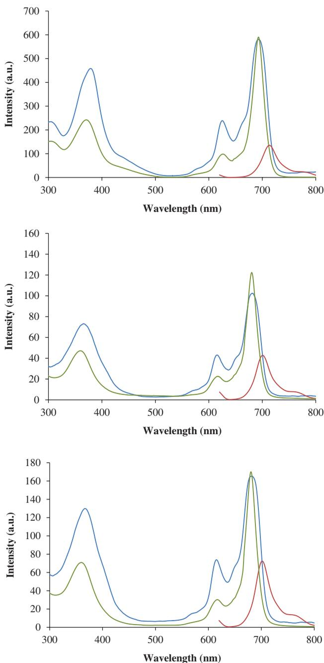
**Figure 7.** Absorption (top), excitation (middle), and emission (bottom) spectra for **3**, **6** and **7** in DMF; excitation wavelength is 614 nm.
