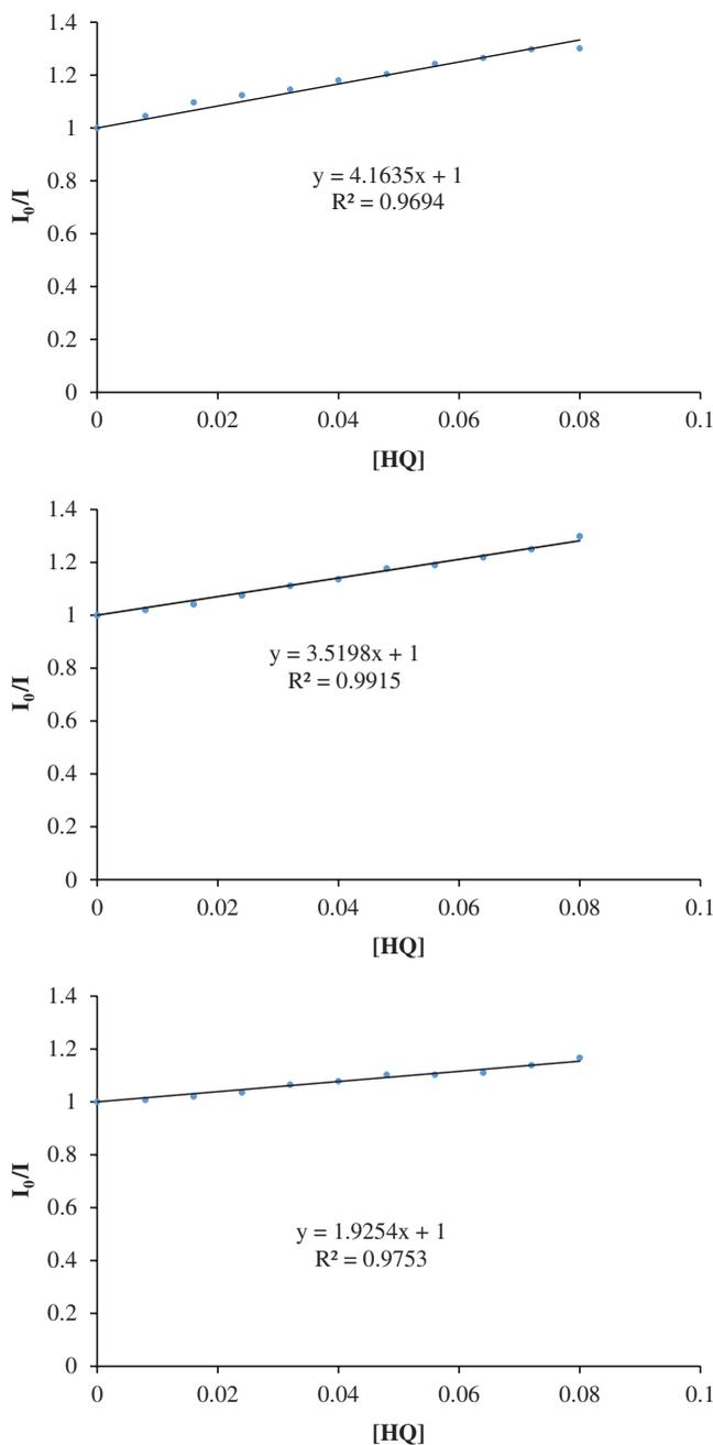
**Figure 9b.** Stern-Volmer plots of **3**, **6**, and **7** quenched by HQ.  $[ZnPc] = 4.00 \mu\text{mol dm}^{-3}$  in DMF. Concentration of the quencher is 0.000, 0.008, 0.016, 0.024, 0.032 and 0.040 mol  $\text{dm}^{-3}$ .
