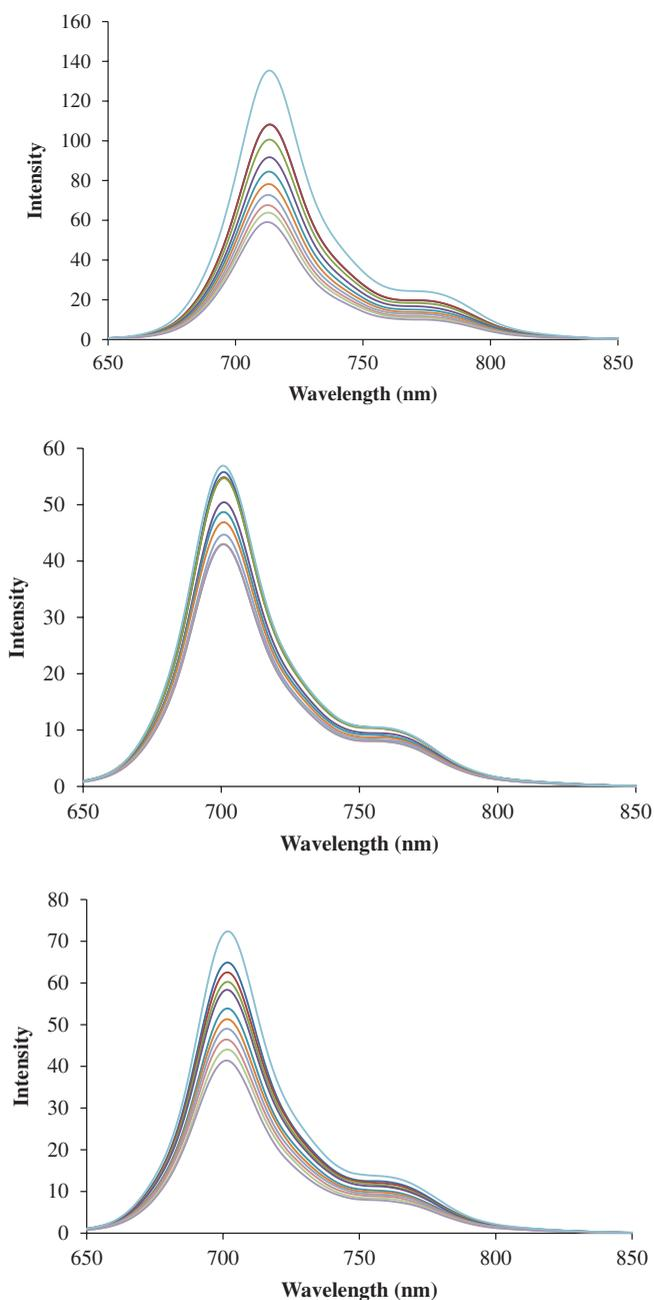
**Figure 8a.** Fluorescent emission spectral changes of **3**, **6**, and **7** ( $4.00 \mu\text{mol dm}^{-3}$ ) in which different concentrations of benzoquinone in DMF was added as quencher. The concentration of benzoquinone is 0.000, 0.008, 0.016, 0.024, 0.032, and 0.040  $\text{mol dm}^{-3}$ .
