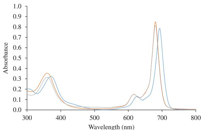
**Figure 6.** Electronic spectra of the zinc phthalocyanine derivatives (**3**, **6**, and **7**) in DMF. The concentration in this study is  $4.00 \mu\text{mol dm}^{-3}$ .
