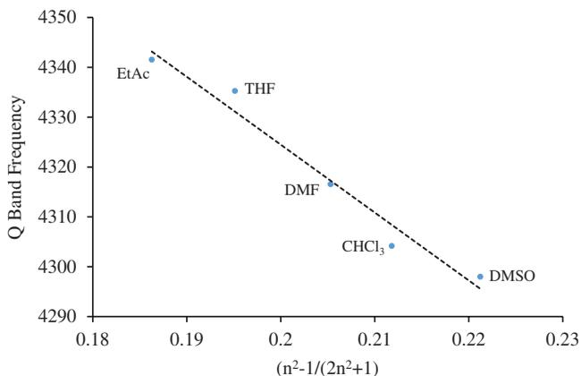
**Figure 5.** Plot of the Q band frequency of ZnPc (**3**) against  $(n^2-1)/(2n^2+1)$ , where  $n$  is the refractive index of the solvent.
