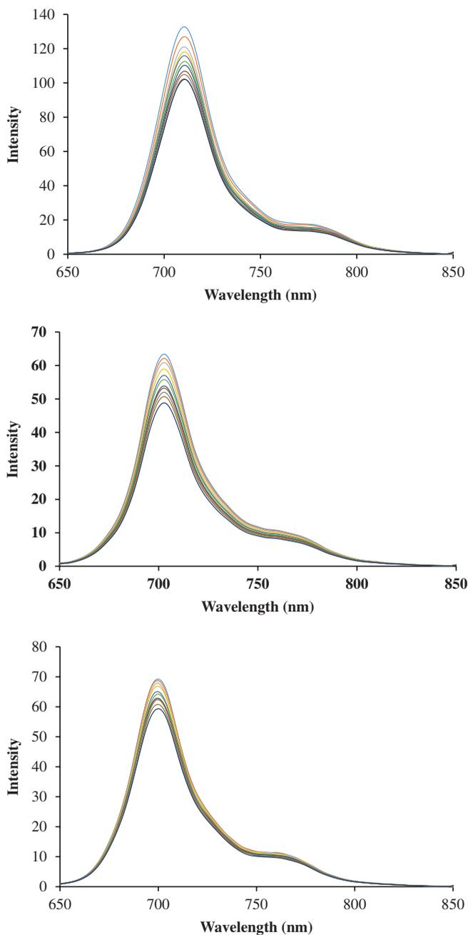
**Figure 8b.** Fluorescent emission spectral changes of **3**, **6**, and **7** ( $4.00 \mu\text{mol dm}^{-3}$ ) in which different concentrations of hydroquinone in DMF was added as quencher. The concentration of hydroquinone is 0.000, 0.008, 0.016, 0.024, 0.032, and 0.040  $\text{mol dm}^{-3}$ .
