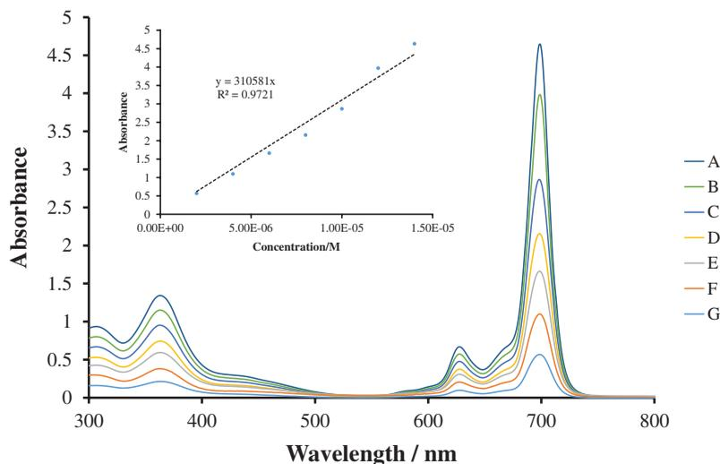
**Figure 3.** Absorption spectra of ZnPc (**3**) in  $\text{CHCl}_3$  at different concentrations:  $14 \times 10^{-6}$  (A),  $12 \times 10^{-6}$  (B),  $10 \times 10^{-6}$  (C),  $8 \times 10^{-6}$  (D),  $6 \times 10^{-6}$  (E) and  $4 \times 10^{-6}$  (F)  $\text{mol dm}^{-3}$ .
