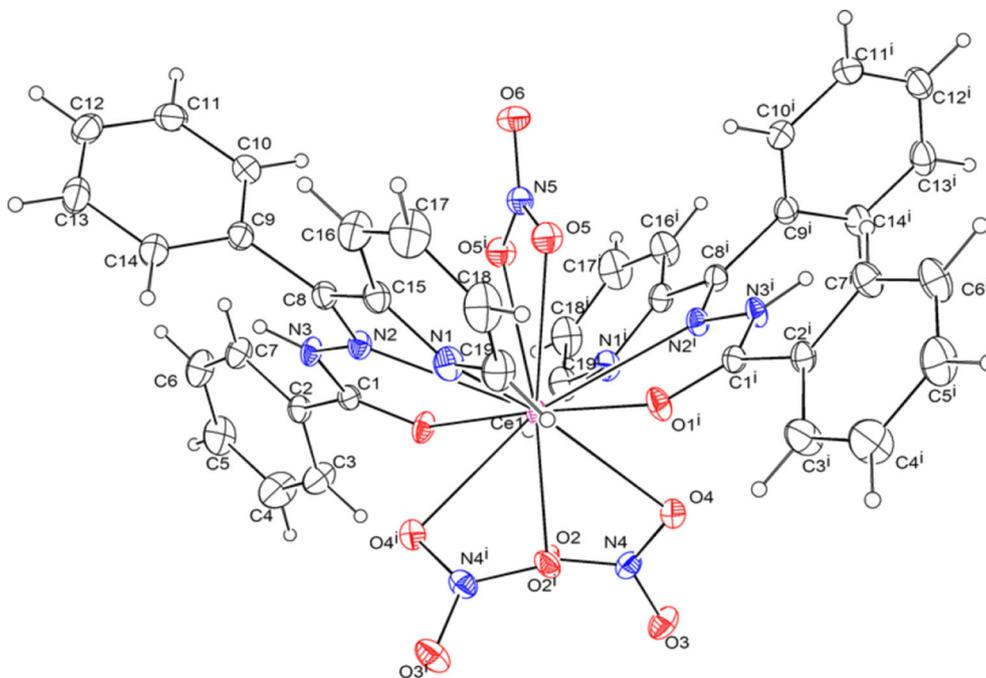
**Figure 2.** ORTEP view showing molecular structure of  $[\text{Ce}(\text{BPBH})_2(\text{NO}_3)_3]$  complex.
