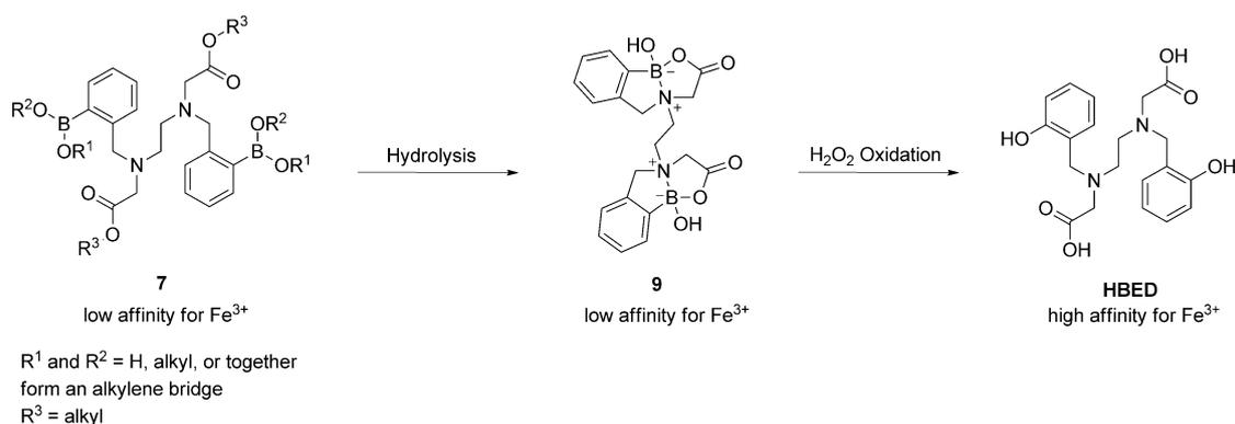
**Scheme 1.** Double prodrugs of the general form **7** undergo activation by nonenzymatic hydrolysis to form **9**, which then is oxidatively deboronated by  $\text{H}_2\text{O}_2$  to generate the parent chelator HBED.
