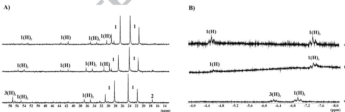
**Fig. 1.** *Operando* (HP) NMR spectra of **1** acquired at 50 °C in different reaction media in the presence of dihydrogen (50 bar): A) <sup>31</sup>P{<sup>1</sup>H} NMR spectra; B) Hydride region of the <sup>1</sup>H NMR spectra: (a) 1:1 (v:v) C<sub>6</sub>D<sub>6</sub>/TFE solvent mixture; (b) 1:1 (v:v) C<sub>6</sub>D<sub>6</sub>/MeOH solvent mixture and (c) neat C<sub>6</sub>D<sub>6</sub>.
