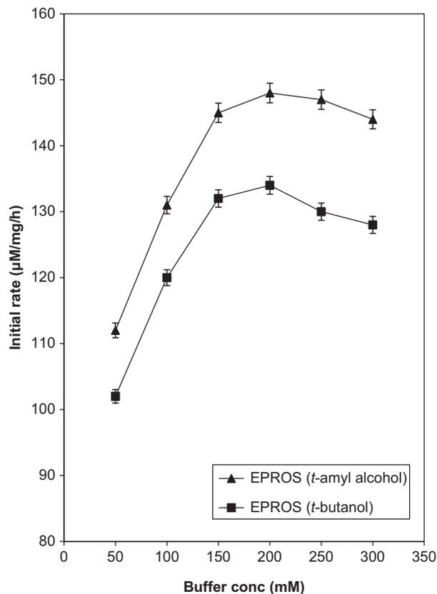
Figure 2. Effect of increase in buffer concentration on the initial rates of EPROS. Reaction conditions were similar to those in Table I and Table II. Each reaction set was run in duplicate and deviations between pairs of experimental data were within 2%.
