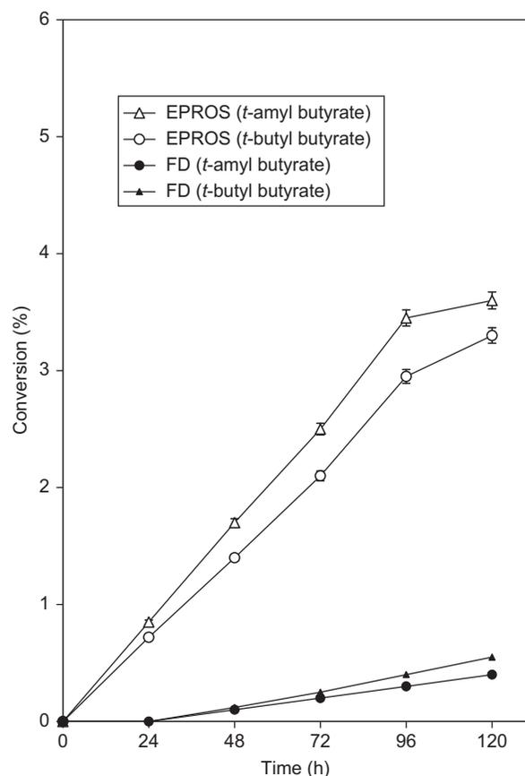
Figure 1. Formation of *tert*-alkylesters by different formulations of *C. rugosa* lipase (prepared in 50 mM phosphate buffer). The conversion (%): The ordinate parameter refers to formation of *t*-alkyl esters only. Reaction conditions were similar to those in Table I and II. Each reaction set was run in duplicate and deviations between pairs of experimental data were within 2%.
