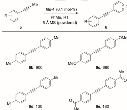
**Scheme 3.** Productivities (TONs) for self-metathesis reactions of *p*-substituted 1-phenyl-1-propynes **5b-e** with **Mo-1**. Reaction conditions: toluene, room temperature, 3 hours, internal standard for GC-MS: *n*-dodecane, 250 mg 5 Å molecular sieves, catalyst:substrate = 1:1000.
