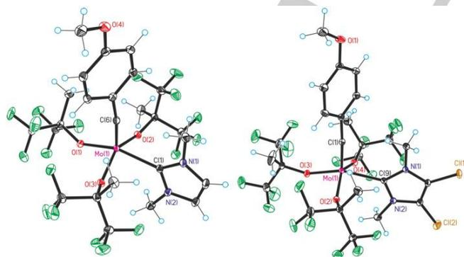
**Figure 2.** Single crystal X-ray structure of **Mo-1** (left) and **Mo-2** (right). Selected bond lengths [pm] for **Mo-1**: Mo(1)-C(6): 173.8(2); Mo(1)-C(1): 224.41(18);  $\tau = 0.18$ <sup>[16]</sup>. Selected bond lengths [pm] for **Mo-2**: Mo(1)-C(1): 174.26(18); Mo(1)-C(9): 225.21(17);  $\tau = 0.24$ .
