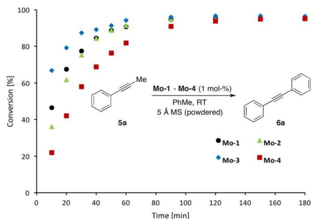
**Figure 4.** Kinetic profiles for the self-metathesis of 1-phenyl-1-propyne with **Mo-1 – Mo-4** at room temperature (see S.I. for further details).
