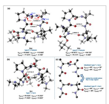
Figure 1: Structural diversity in the X-ray crystal structures of 3. (a) Conformers 3(a) and 3(b) are both consistent with type II'  $\beta$ -hairpin geometries. (b) Conformer 3(c) is consistent with a distorted type I'  $\beta$ -turn. (c) Idealized type I' and II'  $\beta$ -turns as classified by the  $\phi$  and  $\psi$  dihedral angles of the loop residues.  $^{3,10}$
