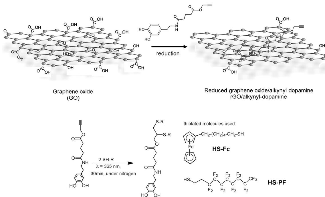
Figure 1. Top: Schematic illustration of the formation of rGO/alkynyl-dopamine nanosheets. Bottom: Reaction of the alkyne-dopamine with thiols by the thiol-yne radical-addition mechanism.
