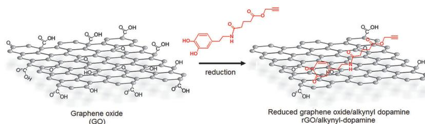
**Modified graphene oxide:** A simple method has been developed for the simultaneous exfoliation and reduction of graphene oxide (GO) to reduced GO (rGO) by using alkyne-terminated dopamine as the reducing agent. The reaction was performed under
