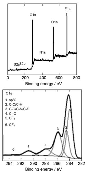
Figure 5. Top: XPS survey spectrum of rGO/alkynyl-dopamine deposited onto ITO after immersion in 10 mM 1*H*,1*H*,2*H*,2*H*-perfluorodecanethiol and UV light irradiation at 365 nm for 30 min at room temperature ( $P=100\text{ mW cm}^{-2}$ ). Bottom: C1s core-level XPS spectrum after thiol-yne reaction with HS-PF.
