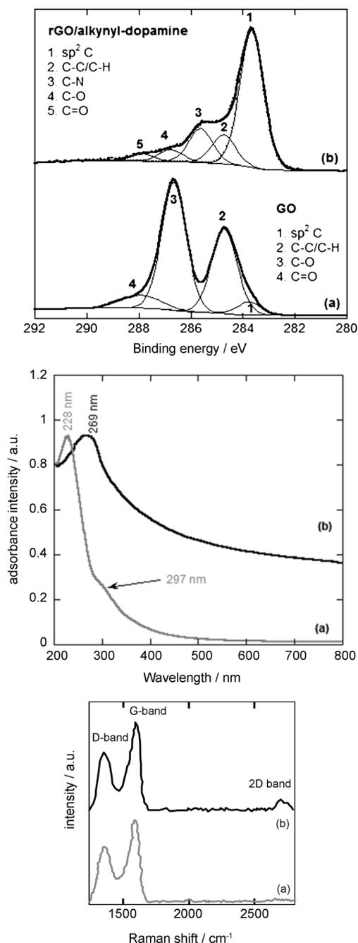
Figure 2. Top: C 1s core-level XPS spectra of GO a) before and b) after reaction with alkynyl-dopamine. Middle: UV/Vis spectra of a) GO in water and b) rGO/alkynyl-dopamine in THF. Bottom: Raman spectra of a) GO and b) rGO/alkynyl-dopamine.
