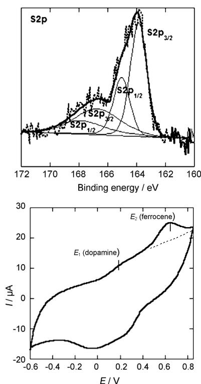
Figure 4. Top: S2p high-resolution XPS spectrum of rGO/alkynyl-dopamine after photochemical reaction ( $\lambda = 365\text{ nm}$ ) with 10 mM 6-ferrocenylhexanethiol for 30 min at room temperature ( $P = 100\text{ mW cm}^{-2}$ ). Bottom: CV of the ITO interface modified with rGO/alkynyl-dopamine after photochemical reaction with 10 mM 6-ferrocenylhexanethiol in 0.1 M PBS (scan rate =  $0.05\text{ V s}^{-1}$ ).
