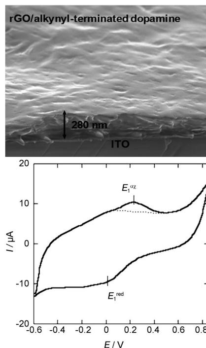
Figure 3. Top: SEM image of an ITO/graphene/alkynyl-dopamine electrode formed by drop-casting (thickness = 280 nm). Bottom: Cyclic voltammogram of an ITO electrode modified by drop-casting with rGO/alkynyl-dopamine in 0.1 M PBS (scan rate = 0.05 V s<sup>-1</sup>).
