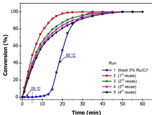
**Fig. 2** Reusing 5% ruthenium on carbon in the hydrogenation of 1-methylpyrrole (MP). Conditions: 2.0 g substrate, 50 cm<sup>3</sup> methanol, 0.4 g catalyst, 25 °C, \*25–60 °C, 10 bar
