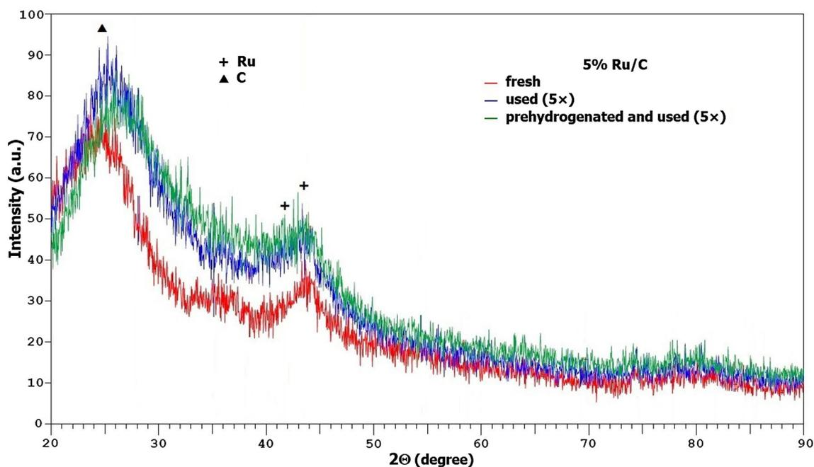
**Fig. 6** XRD patterns of 5% Ru/C catalyst in fresh and used (5 $\times$ ) forms
