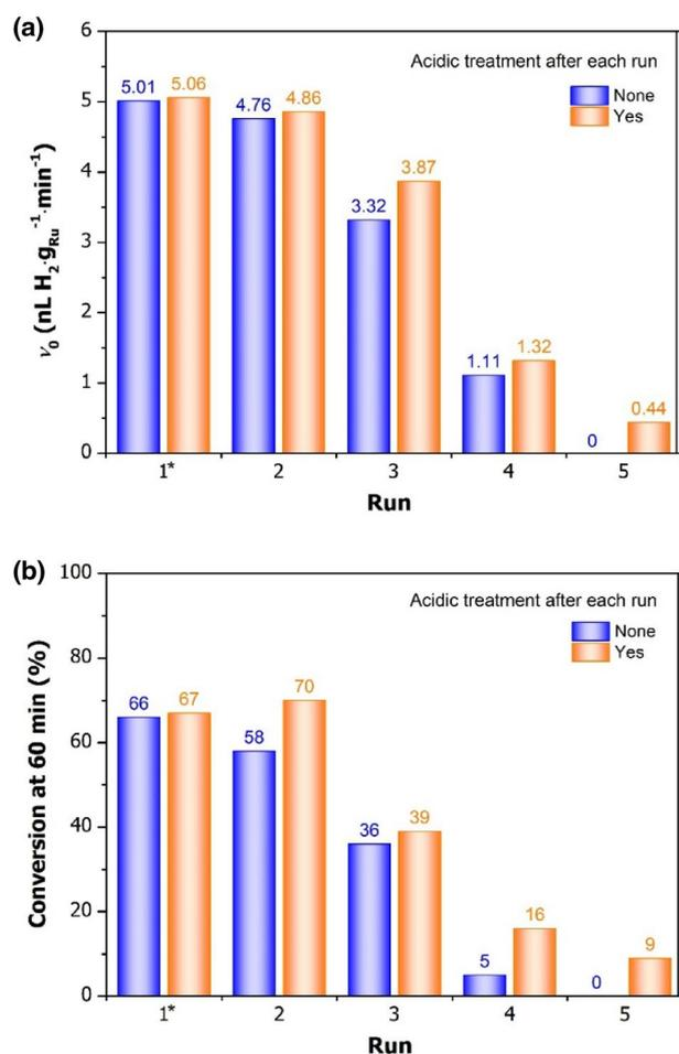
**Fig. 11** Effects of acidic treatment after each run and reuse of the catalyst on the initial rate ( $v_0$ ) (a) and the conversion at 60 min (b) in the hydrogenation of 1-methylpyrrole (MP) over 5% Ru/C. Conditions: 2.0 g substrate, 0.1 g catalyst, 50 cm<sup>3</sup> methanol, 25 °C, \*25–60 °C 10 bar; acidic treatment: 2×5 cm<sup>3</sup> 5% acetic acid, then 2×10 cm<sup>3</sup> distilled water
