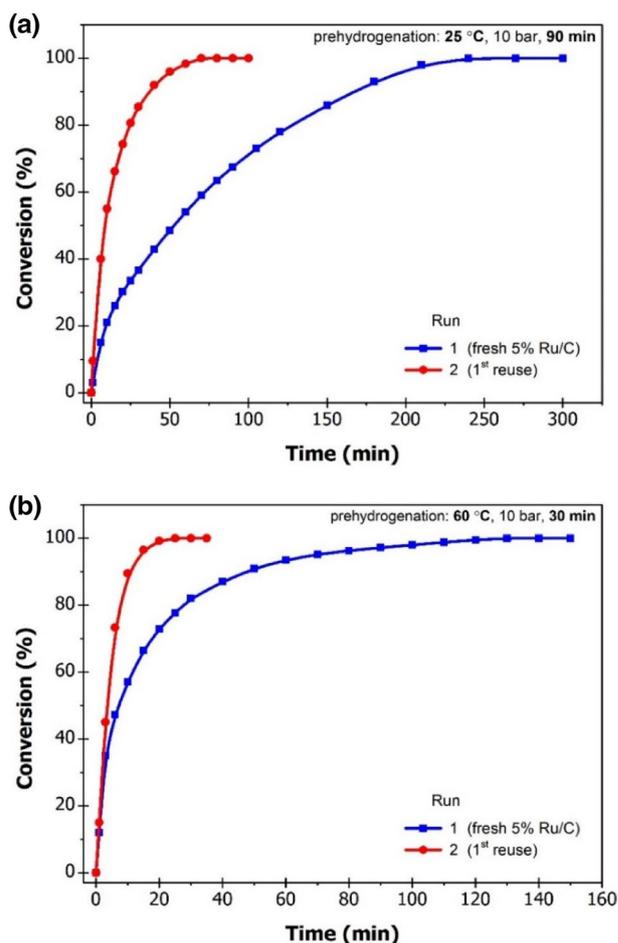
**Fig. 4** Conversion of 1-methylpyrrole (MP) vs. time over 5% Ru/C prehydrogenated at 25 °C and 90 min (a) or at 60 °C and 30 min (b). Conditions: 2.0 g substrate, 50 cm<sup>3</sup> methanol, 0.4 g catalyst, 25 °C, 10 bar; pretreatment: 30 cm<sup>3</sup> methanol, 10 bar
