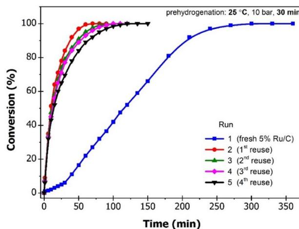
**Fig. 3** Conversion of 1-methylpyrrole (MP) vs. time over 5% Ru/C prehydrogenated at 25 °C. Conditions: 2.0 g substrate, 50 cm<sup>3</sup> methanol, 0.4 g catalyst, 25 °C, 10 bar; pretreatment: 30 cm<sup>3</sup> methanol, 25 °C, 10 bar, 30 min
