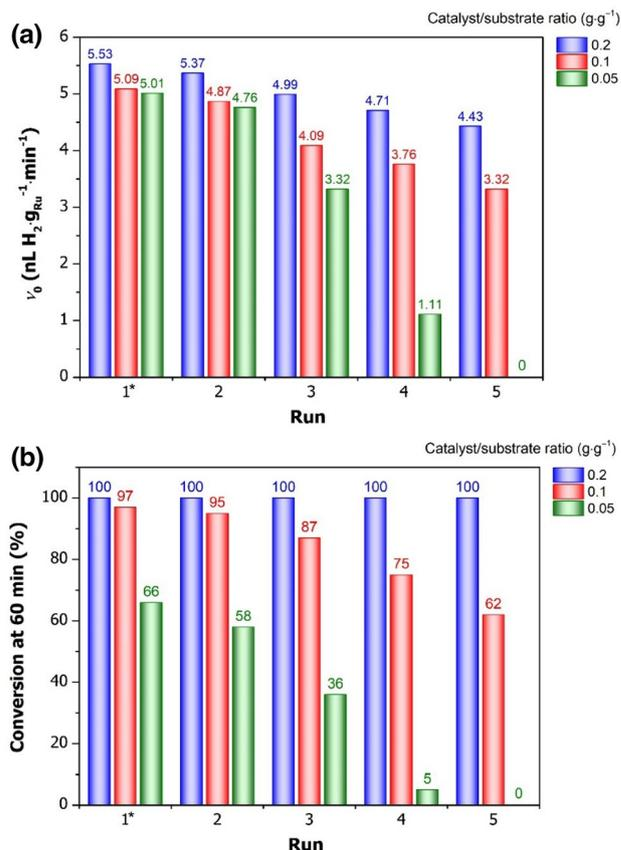
**Fig. 9** Effects of amount and reuse of the catalyst on the initial rate ( $v_0$ ) (a) and the conversion at 60 min (b) in the hydrogenation of 1-methylpyrrole (MP) over 5% Ru/C. Conditions: 2.0 g substrate, 50 cm<sup>3</sup> methanol, 25 °C, \*25–60 °C 10 bar
