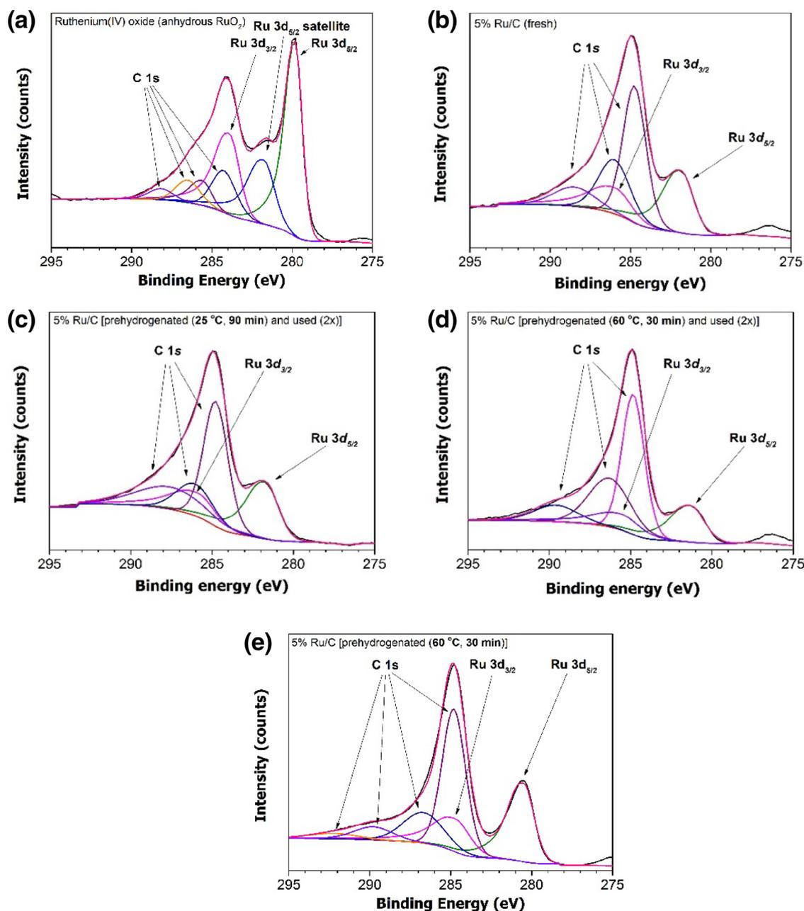
**Fig. 7** High-resolution and deconvolution XP spectra of anhydrous  $\text{RuO}_2$  as a reference (a) and 5% Ru/C catalyst in different forms: fresh (b), prehydrogenated at 25 °C and used (2 $\times$ ) (c), prehydrogenated at
