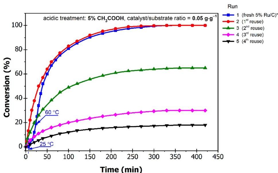
as did in those reactions where 5% ruthenium on carbon was applied without acidic treatment, but better results (65 and 30%, respectively) were achieved. Finally, in the fifth run, a significantly higher conversion value was obtained over the acidic treated catalyst (18%) than using the untreated one (0%).
