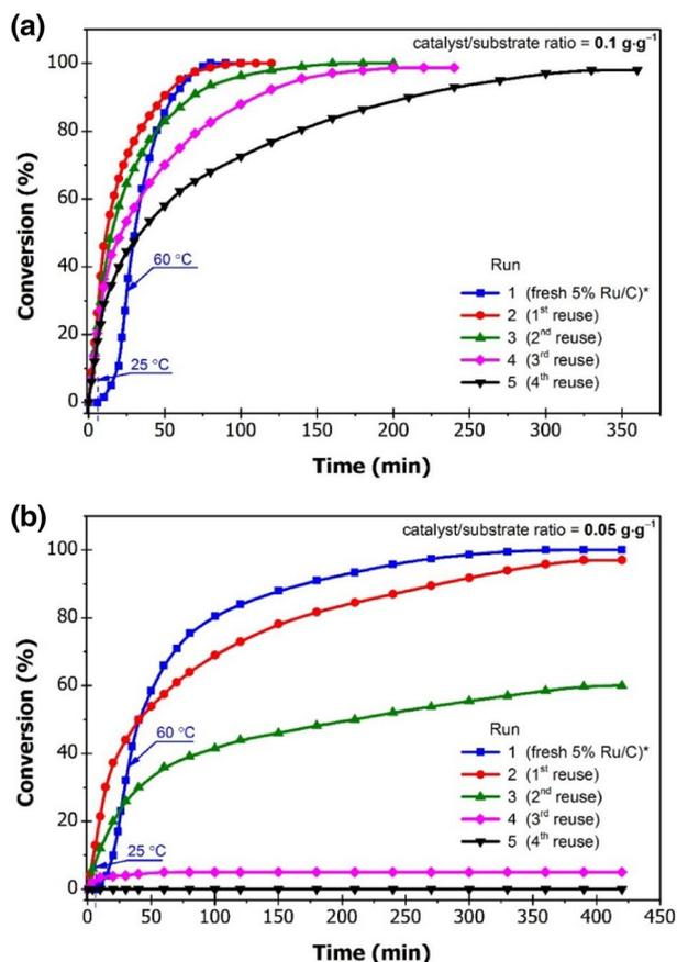
**Fig. 8** Conversion of 1-methylpyrrole (MP) vs. time over 5% Ru/C, at different catalyst/substrate ratios: 0.1 g g<sup>-1</sup> (a) and 0.05 g g<sup>-1</sup> (b). Conditions: 2.0 g substrate, 50 cm<sup>3</sup> methanol, 25 °C, \*25–60 °C 10 bar
