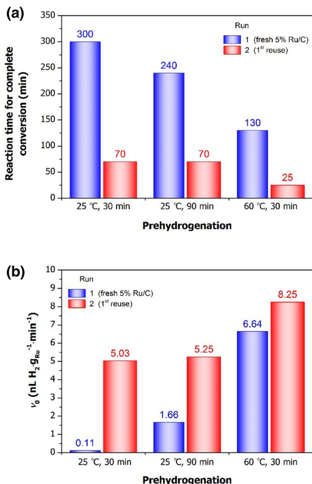
**Fig. 5** Effects of time and temperature of prehydrogenation on the reaction time for complete conversion (a) and the initial rate ( $v_0$ ) (b) in the hydrogenation of MP over prehydrogenated 5% Ru/C. Conditions: 2.0 g substrate, 50 cm<sup>3</sup> methanol, 0.4 g catalyst, 25 °C, 10 bar; pretreatment: 30 cm<sup>3</sup> methanol, 10 bar
