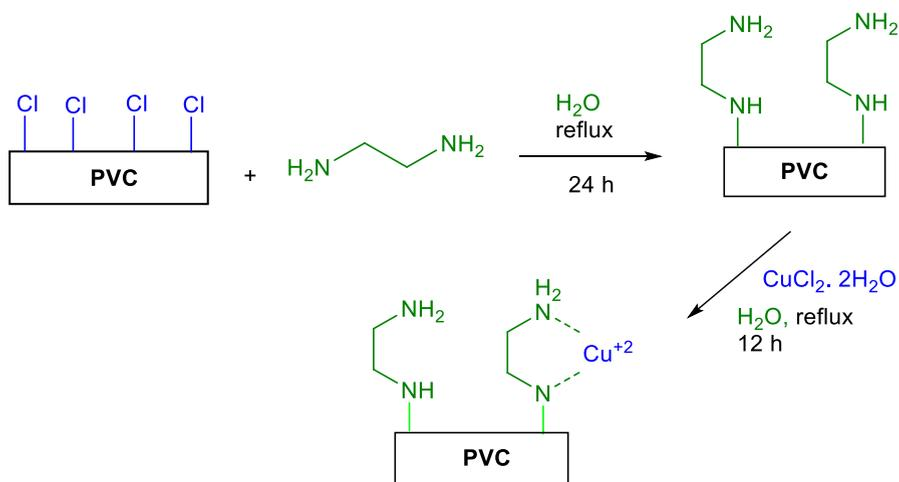
**Scheme 2** Synthesis of PVC-supported ethylenediamine copper(II) complex from PVC, ethylenediamine, and CuCl<sub>2</sub>·2H<sub>2</sub>O
