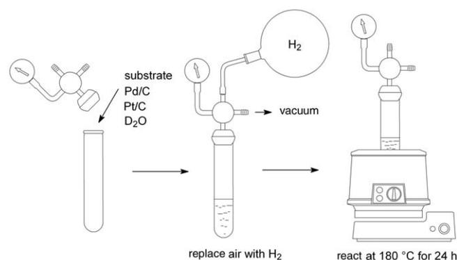
**Figure 1** Typical reaction procedure in a sealed tube.
